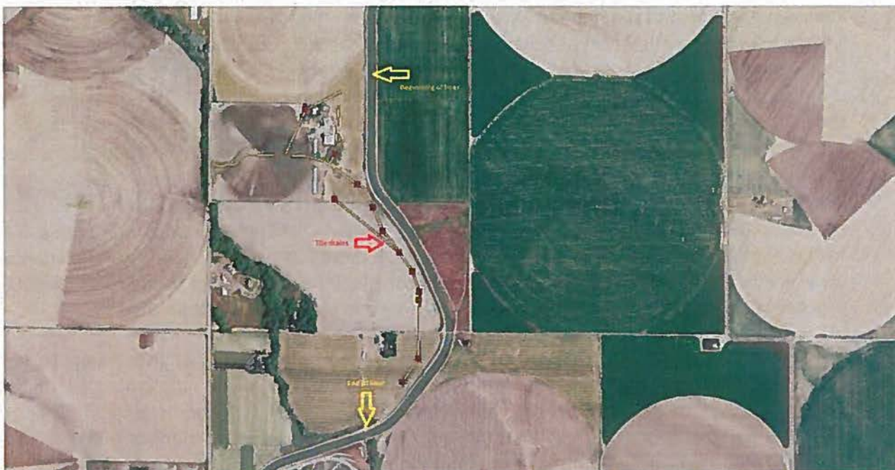
Figure 4. Aerial Image of Project Area Showing Existing Drain Tiles Installed Adjacent to the Canal to Control Groundwater Elevation Due to Canal Seepage Loss
