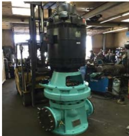
Figure 1-3: Pressure Reducing Turbine
