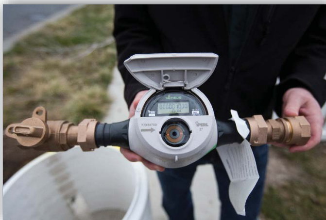
1" Sensus iPERL Secondary Water Meter (Photo courtesy of Standard-Examiner)
