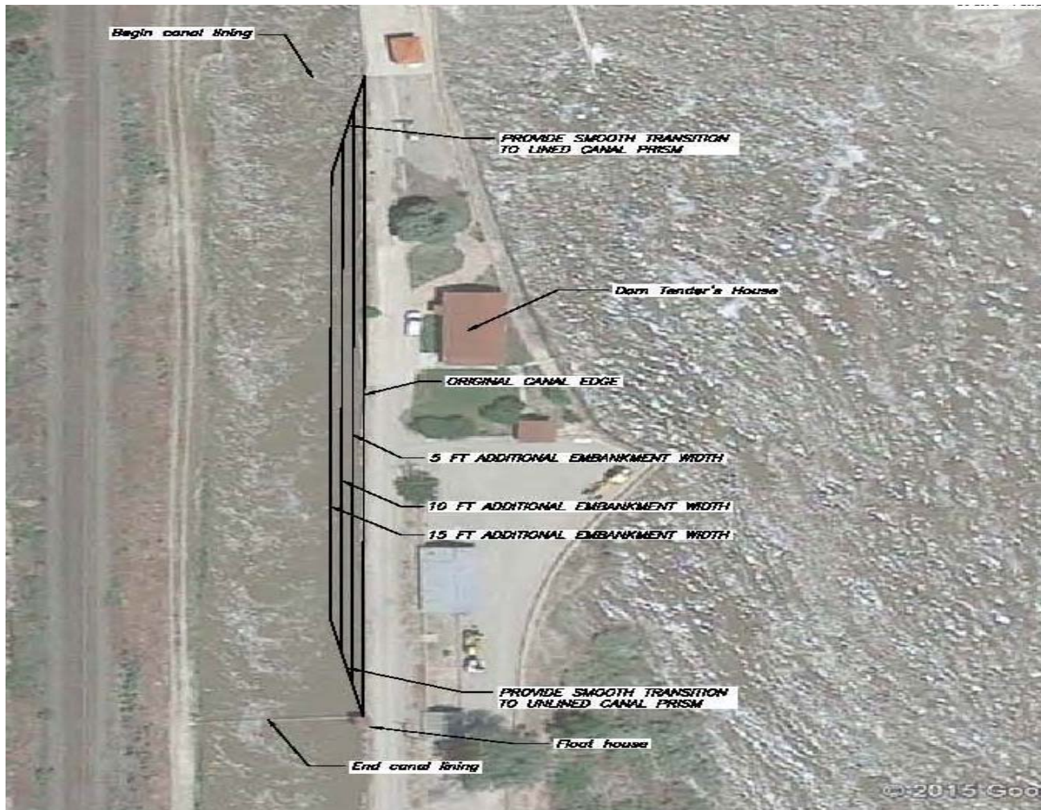
Figure 7. Aerial View of the Canal Section with Varying Widths (Excerpt from Reclamation Drawing, 2015).
