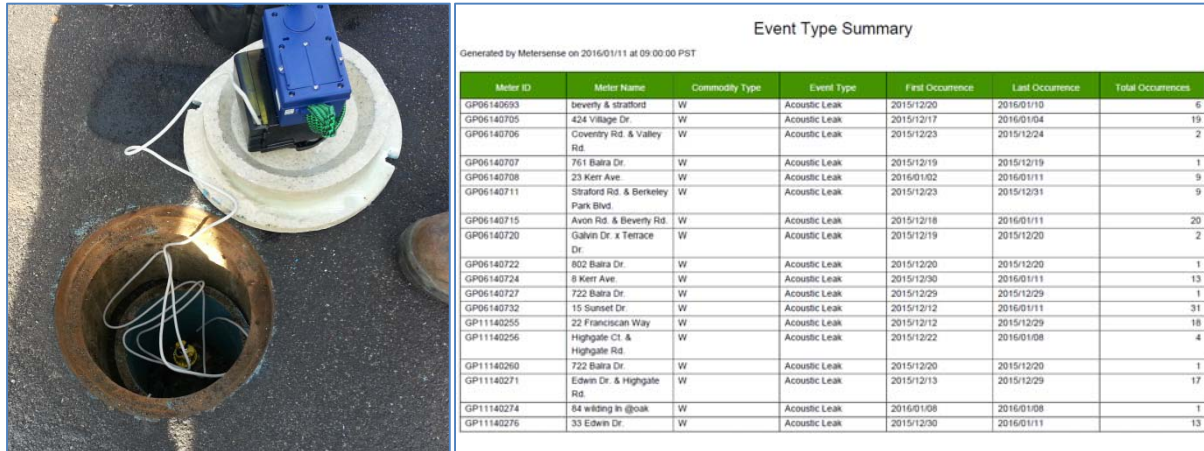
Figures 23 and 24. Fixed Network Leak Detection Pilot Equipment and Sample Report.
