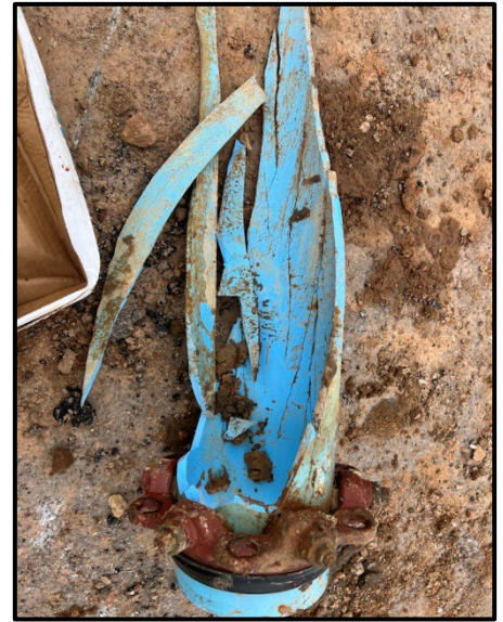
Figure 3: Exploded Pipe Due to Freezing
