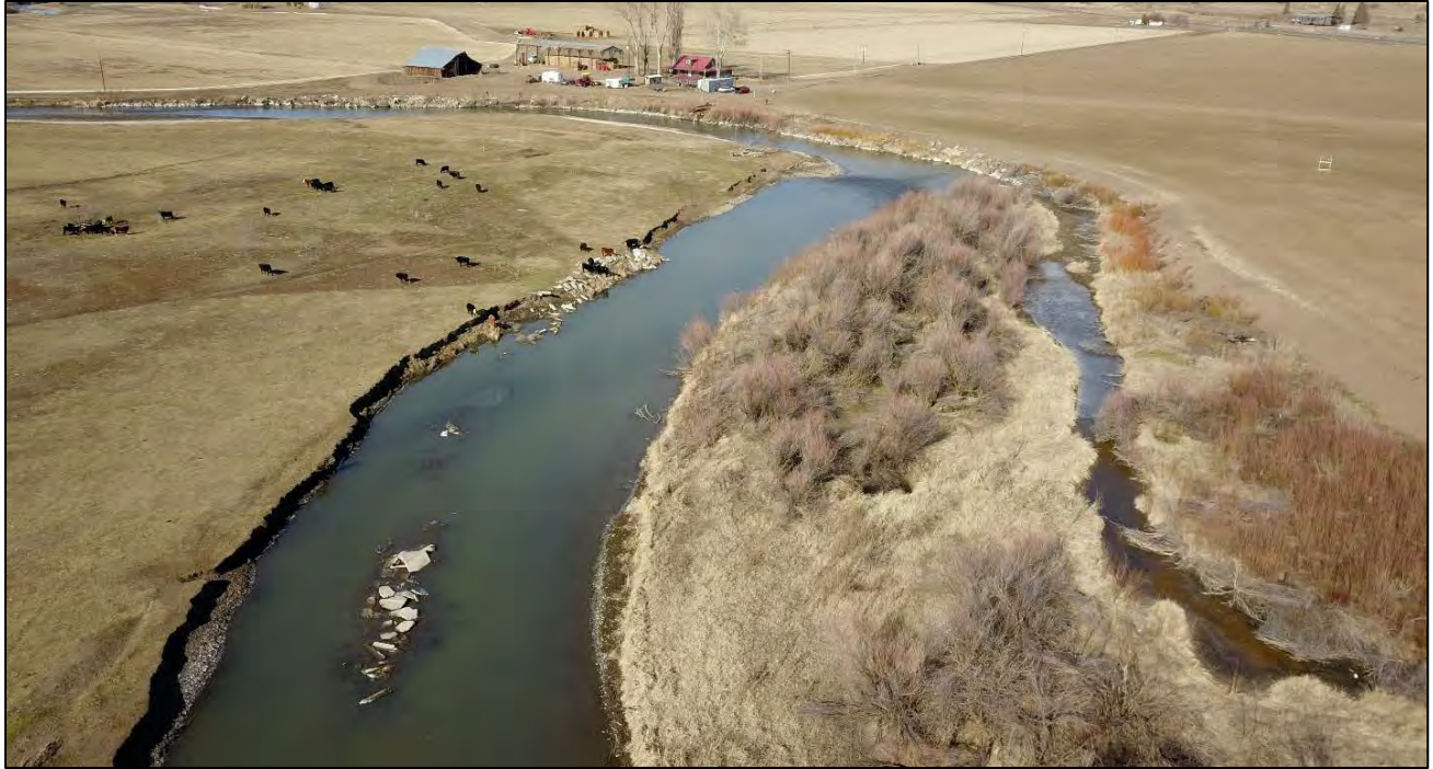
Oblique aerial view looking downstream showing existing upstream side channel at Silva Ranch at low stage when dam bladders were not inflated. The existing side channel will be improved with increased depths and large wood structures. Photo taken February 1, 2022.
