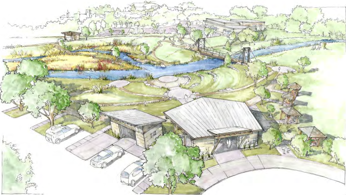
Figure 8. Proposed park concept, looking across the river at the proposed wetland, new side channel and relocated levee.
