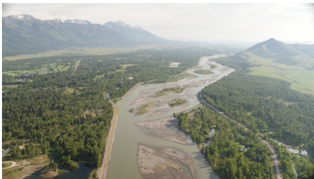
Figure 10: Levee confinement and associated floodplain disconnection along the Snake River
