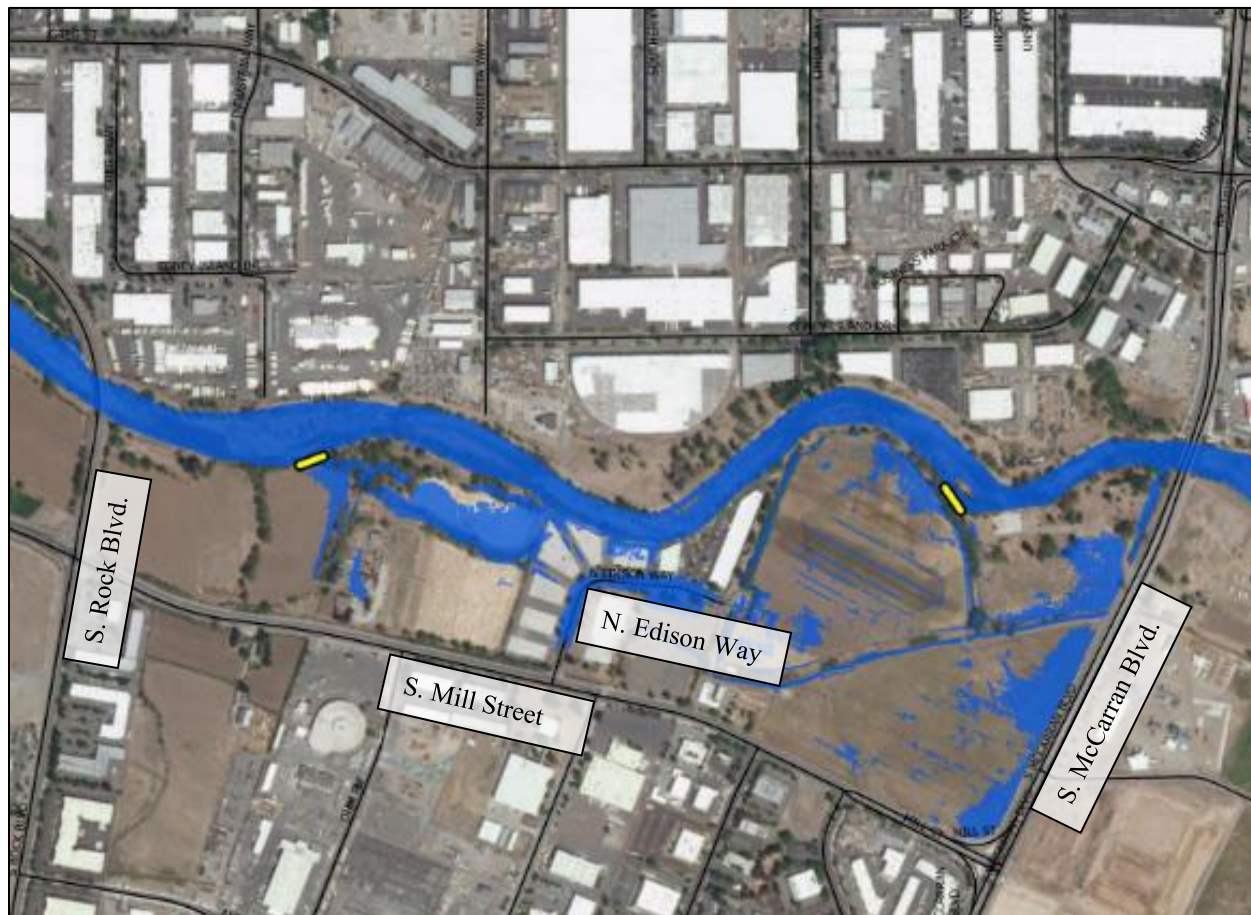
Figure 20.—Truckee River Truckee Meadows Reach, 6,000-cfs Peak Flow Inundation Boundary for Channel Capacity Analysis. Blue shading indicates areas inundated in the 2D HEC-RAS during the routing of the 6,000-cfs peak flow synthetic hydrograph, and the yellow lines indicate breakout locations.
