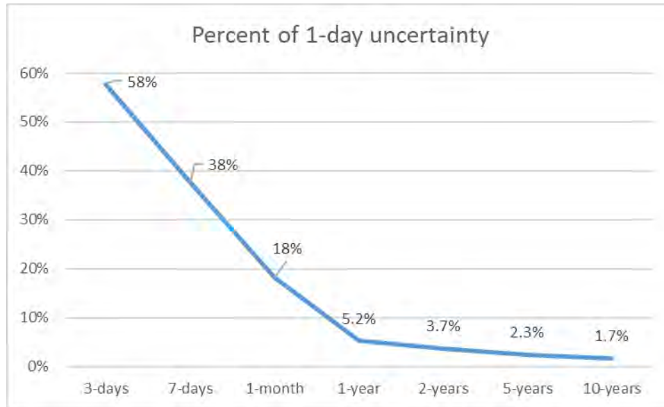
Figure 34 Plot that shows the reduction in random uncertainty compared to the one-day uncertainty if the same average value were computed over lengthening time periods. Uncertainty decreases with the duration ( N ) of the experiment by 1/\sqrt{N} . (Maidment, 1993, p. 13.11)
