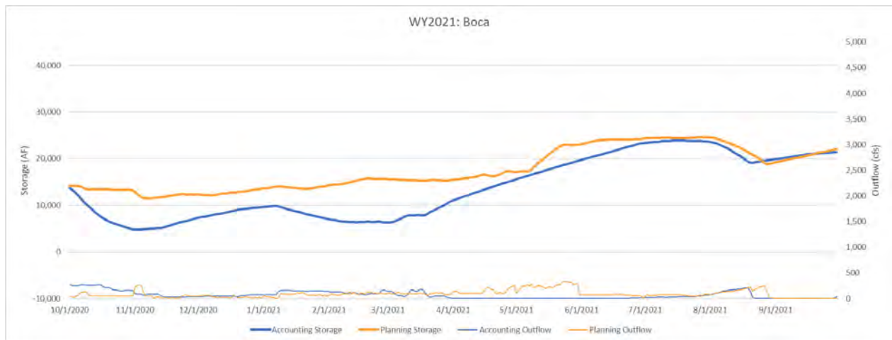
Figure 113. WY 2021 Boca Reservoir Outflow (right axis) and Storage (left axis) results from the Accounting (blue) and Planning Models (orange).
