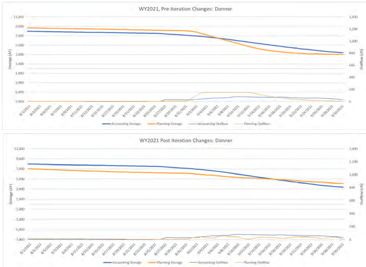
Figure 44. WY 2021 Donner Lake Storage and Outflow results in the Accounting Model (blue) and Planning Model (orange) prior to the Iteration 1 changes to the Planning Model (top) and after Iteration 1 changes to the Planning Model
