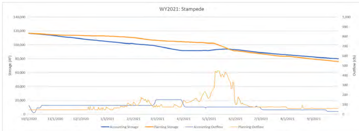
Figure 4. Accounting (blue) and Planning (orange) Model Stampedede Reservoir Storage comparison for WY 2021.
