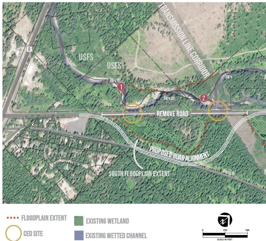
Figure 5, Depiction of the road realignment concept and the location of the two Washington State Department of Transportation Chronic Environmental Deficiency sites along Nason Creek, 2021.
