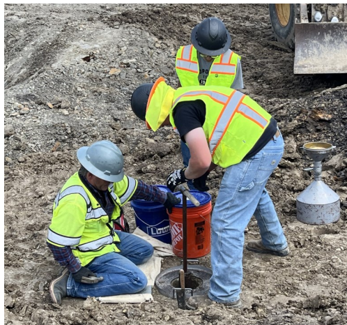
FCCO employees-Brad Gordanier, Kevin Drechsel and Isaiah Smith conduct a sand cone density test. Reclamation photo by Paul Bergstrom
