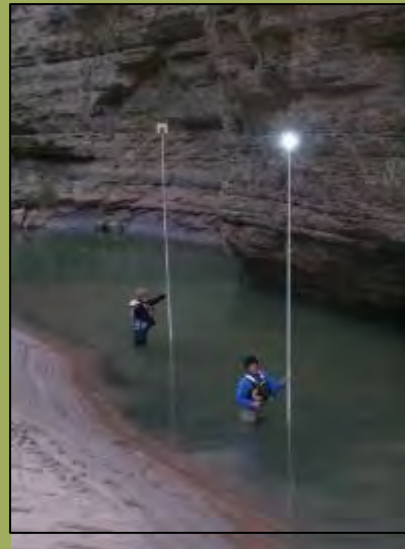
Data collection: old school total station and survey rod
