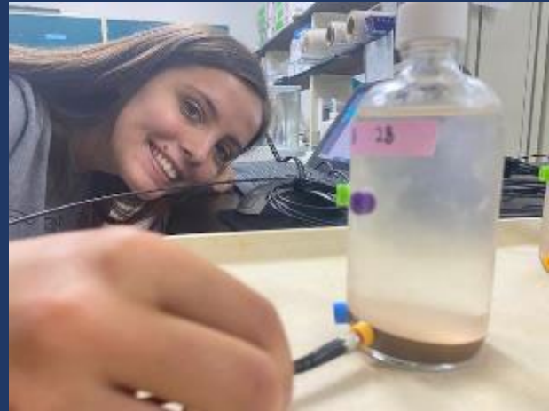
Anna Fatta measures dissolved oxygen and pH in a closed bottle incubation.
