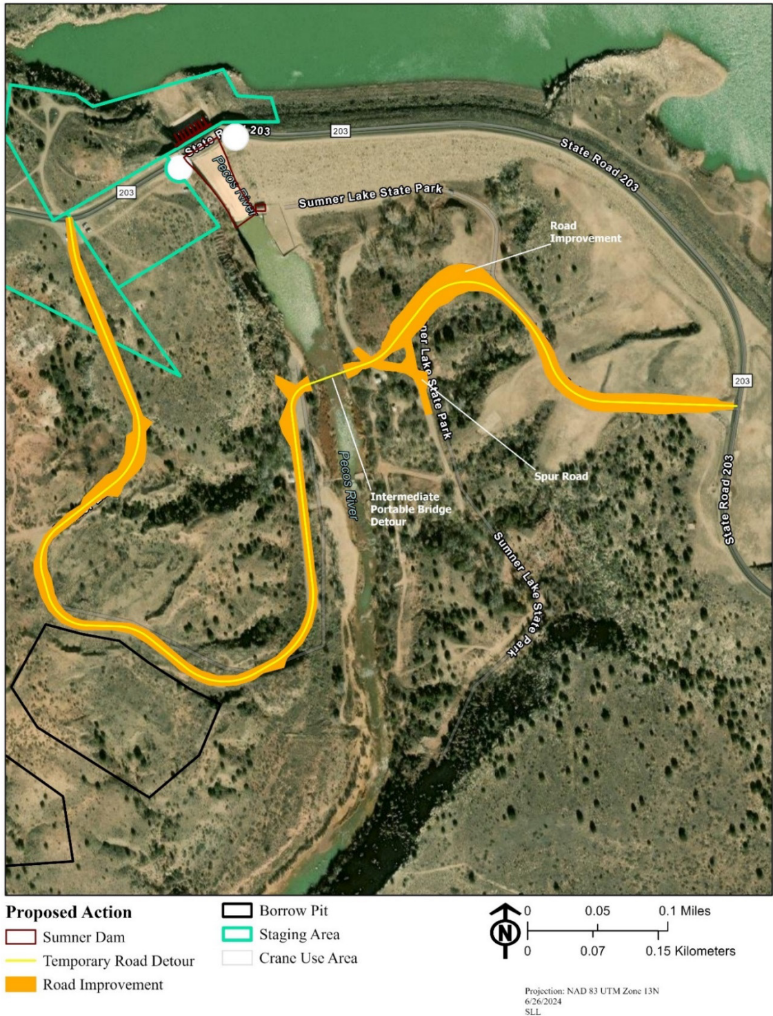
Figure 3. Road Improvements for Intermediate Access Route.
