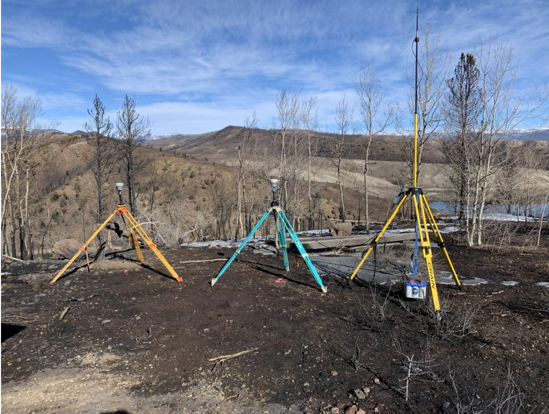
Figure 9. Photograph of GPS base stations used by River Science and Reclamation during the November 2020 survey.
