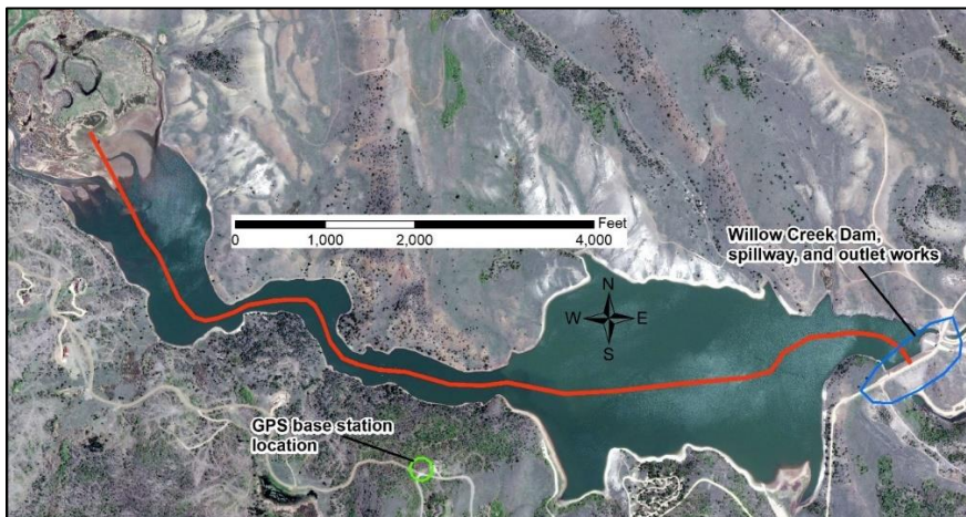
Figure 2 Aerial photograph of Willow Creek Reservoir showing the centerline profile and GPS base station location.
