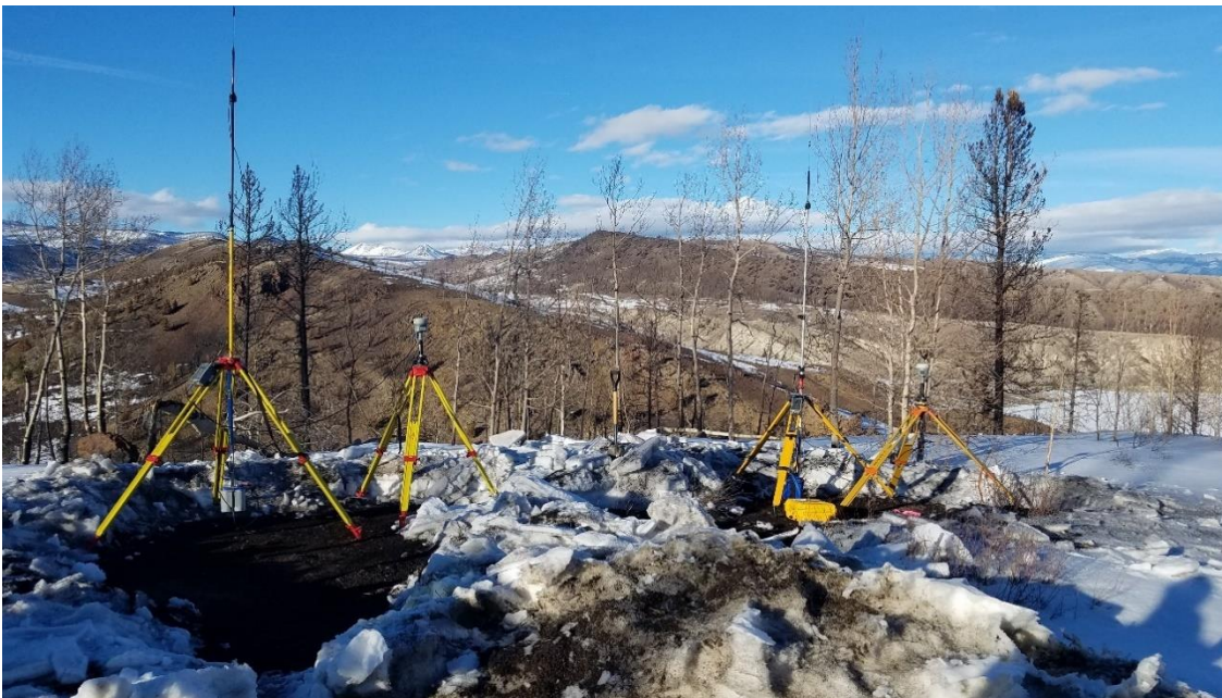
Figure 10. Photograph of GPS base stations used by River Science and Reclamation during the February 2021 survey.
