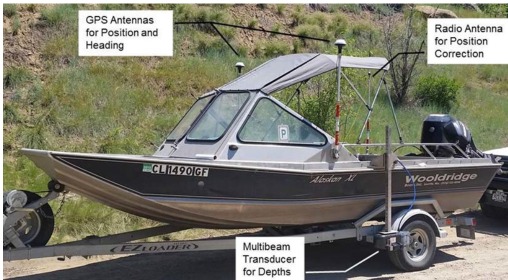
Figure 15. Wooldridge boat with RTK-GPS and multibeam depth sounder system.
