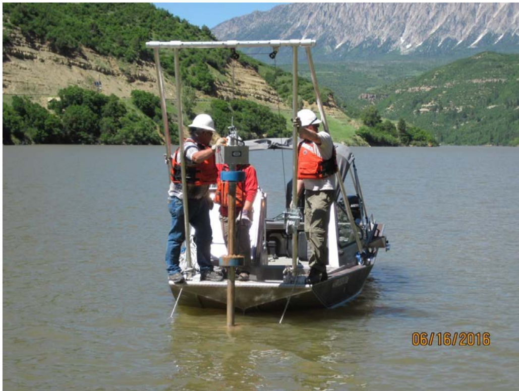
Figure 10.—VibeCore sampling configuration mounted to Wooldridge boat used to collect sediment samples at Paonia Reservoir in Colorado. No photo available of boat deployed at Shadow Mountain Reservoir.
