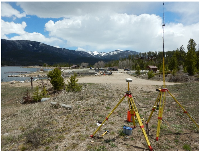
Figure A-2.—The RTK-GPS base station set-up used during the survey of Shadow Mountain Reservoir in Colorado is typical of the set up used for other reservoir surveys.
