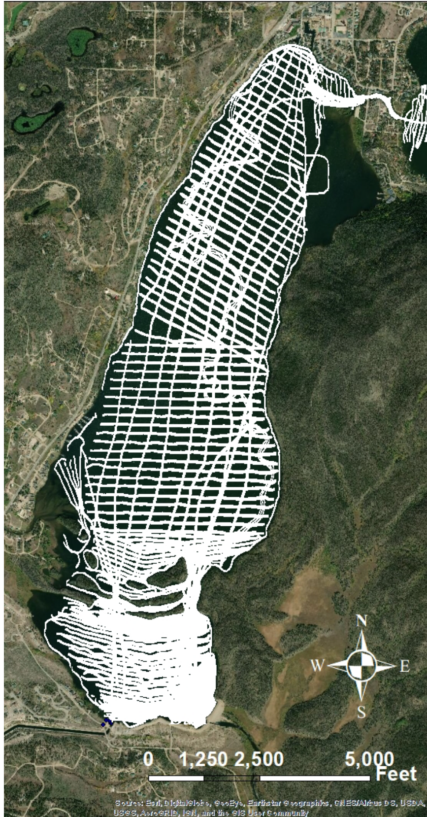
Figure 7.—Map of bathymetric survey data coverage.
