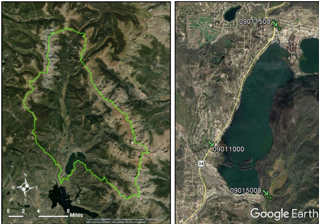
Figure 2.—The watershed above Shadow Mountain Dam has a total drainage area of 186 mi 2 (left). Three USGS gages (not all still active) used to estimate mean inflow and outflow rates (right).
