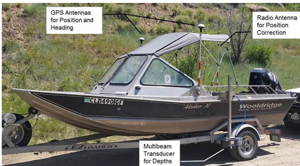
Figure 24. Wooldridge boat with RTK-GPS and multibeam depth sounder system.
