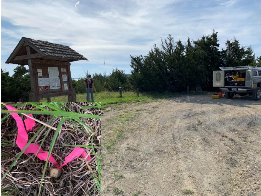
Figure 13. GPS base and temporary monument (inset photo) located in pull-out on dirt road along south side of reservoir.
