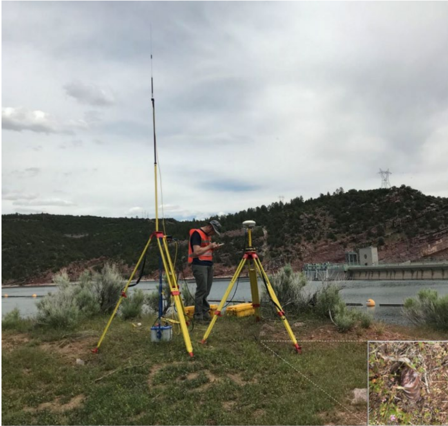
Figure A-3. The RTK-GPS base station set-up used during the survey Clark Canyon Reservoir in Montana is typical of the set up used for other reservoir surveys.
