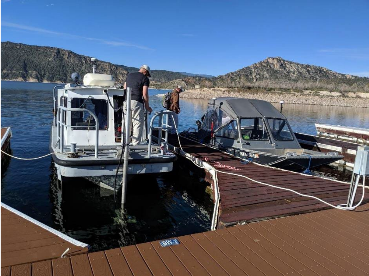
Figure A-2. Both survey vessels with multibeam systems mounted during the 2019 bathymetric data collection. The SeaArk is on the left with the Wooldridge on the right of the photo
