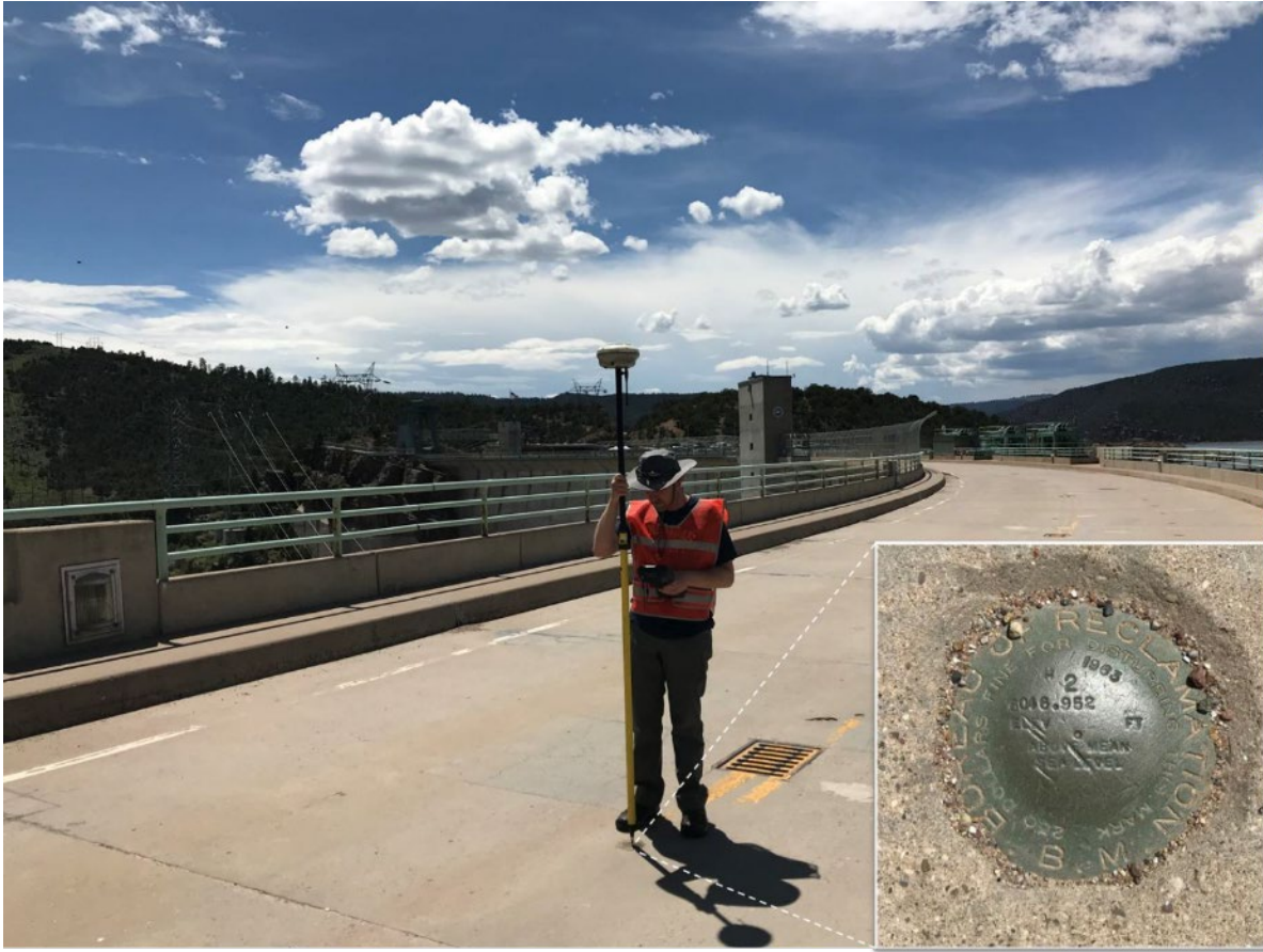
Figure 13. RTK GPS measurement of one of the brass caps located on the dam crest used to vertically reference bathymetry data to RPVD
