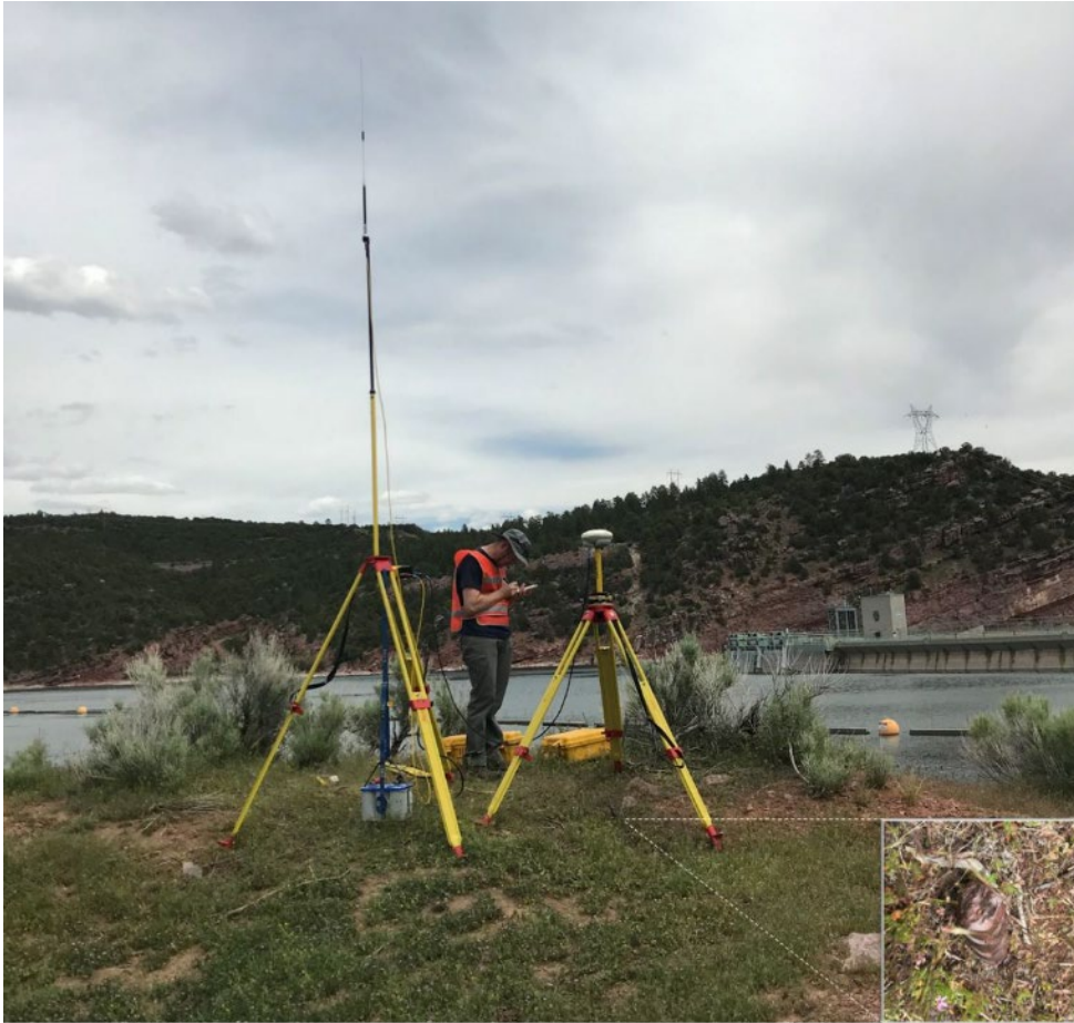
Figure 12. RTK GPS base station used to measure water surface elevations near the dam and control points on the dam to reference bathymetric survey vertical datum to RPVD
