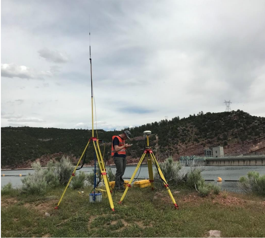
Figure 17. The RTK-GPS base station set-up used during the survey of Flaming Gorge Reservoir in Utah and Wyoming is typical of the set up used for other reservoir surveys.
