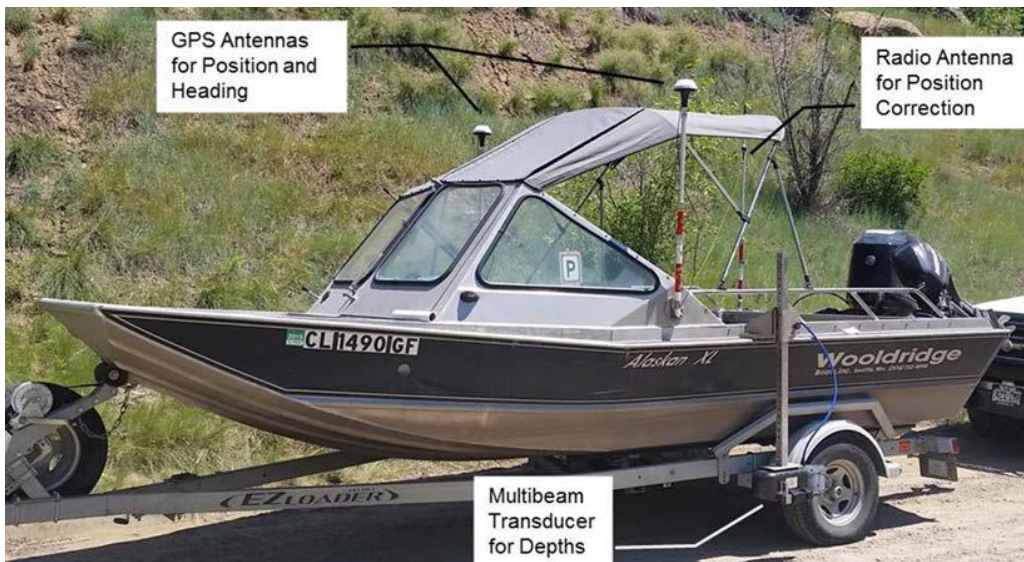
Figure 15. Wooldridge boat with GPS and multibeam depth sounder system.
