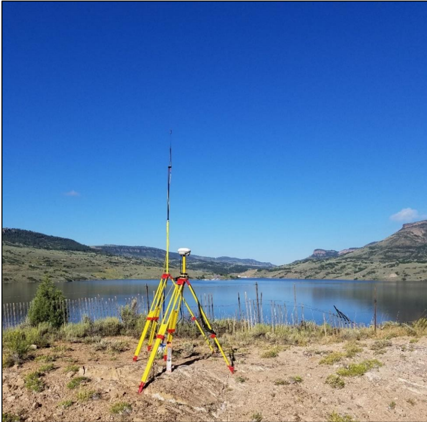
Figure A-2. The RTK-GPS base station set-up used during the Blue Mesa Reservoir survey (NGS bench mark designation S424 near Sapinero, Colorado is shown).
