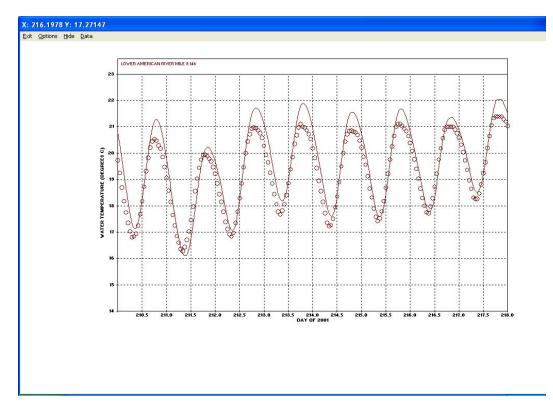
**Figure 1**.—Example of closeness-of-fit between model (line) and observed (circles) daily water temperature data at one riverine location (from Bender et al, 2007).
