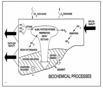
**Figure 3**.—Major biochemical processes modeled in reservoirs (Bender et al, 1990)
