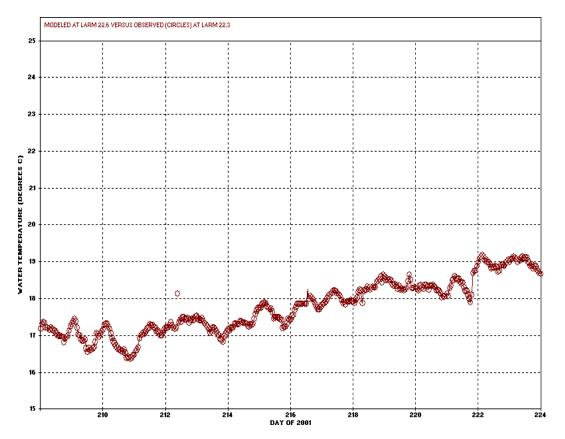
**Figure 6**.—Modeled (line) and instantaneous observed (circles) release temperature versus time near Nimbus Dam at Hazel Avenue Bridge (CDEC sample site AHZ-LARM 22.3 miles from mouth) from July 27, 2001 to August 12, 2001, Bender et al, 2007.
