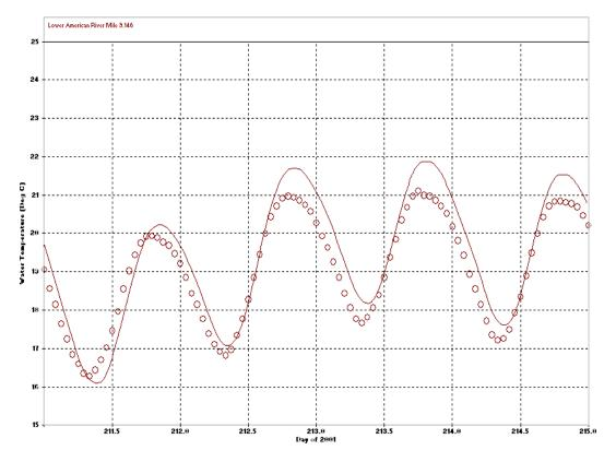
**Figure 5**.—Modeled (line) and instantaneous observed (circles) temperatures versus time at Watt Avenue Bridge (9.146 miles from mouth) during July 30, 2001, through August 3, 2001 (temperature in °C versus day of year), Bender et al, 2007.
