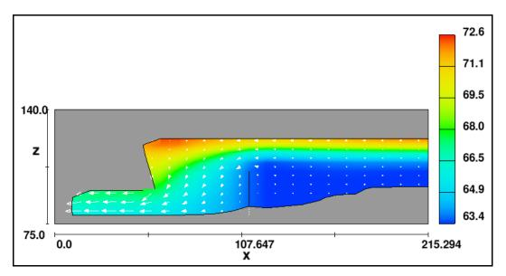
**Figure 4**.—Modeled temperature contours upstream and downstream of a debris barrier wall in near-field of power plant intakes into a dam (flow direction is right to left). The color contours represent temperature (in degrees Fahrenheit (°F)), x and z distances are in feet, and vectors represent resultant velocities (Bender, et al, 2007).
