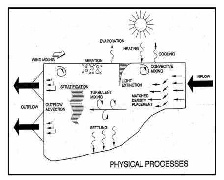
**Figure 2**.—Major physical processes modeled in reservoirs (Bender et al., 1990)
