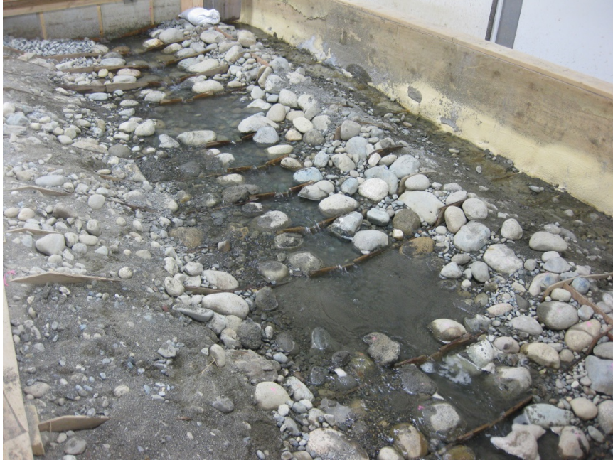
Figure 1. Physical hydraulic model (1:6 scale) of a section of the proposed Trabuco Creek fishway design at Northwest Hydraulic Consultants hydraulics laboratory in Seattle, WA.
