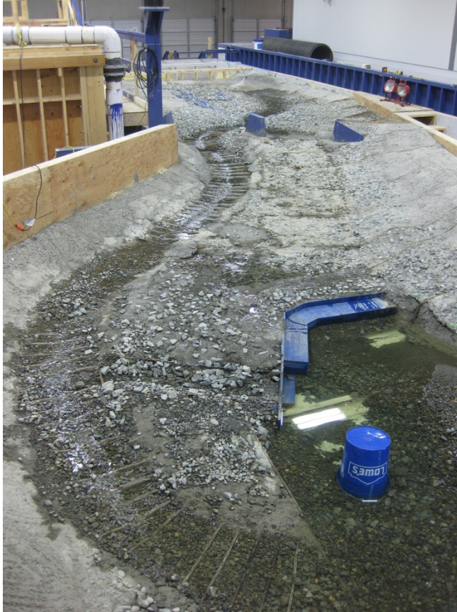
Figure 2. Physical hydraulic model (1:20 scale) of the proposed Trabuco Creek fishway design at Northwest Hydraulic Consultants hydraulics laboratory in Seattle, WA.
