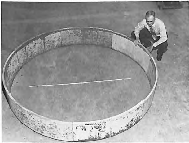
Cylindrical precast concrete segments form an 8-foot internal-diameter support and lining system.
