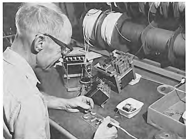
Prototype reactor relay assembled in the E&R Center laboratory.
