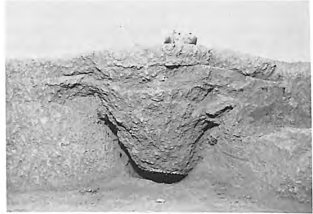
Failure shape formed by uplift loads on 1/6-scale model of belled auger transmission tower footing.
