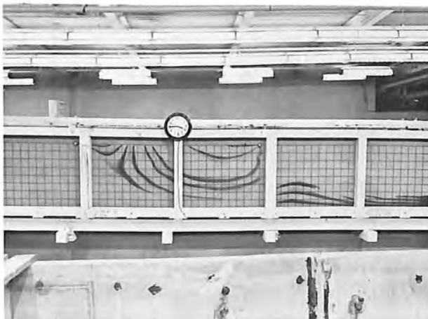
Dye tracers photographed in a sand tank flume with the ground surface sloping 2½ percent.
