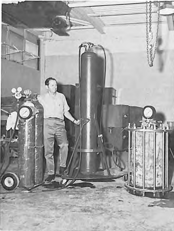
Hydrostatic testing of polymer-impregnated concrete pipe.
