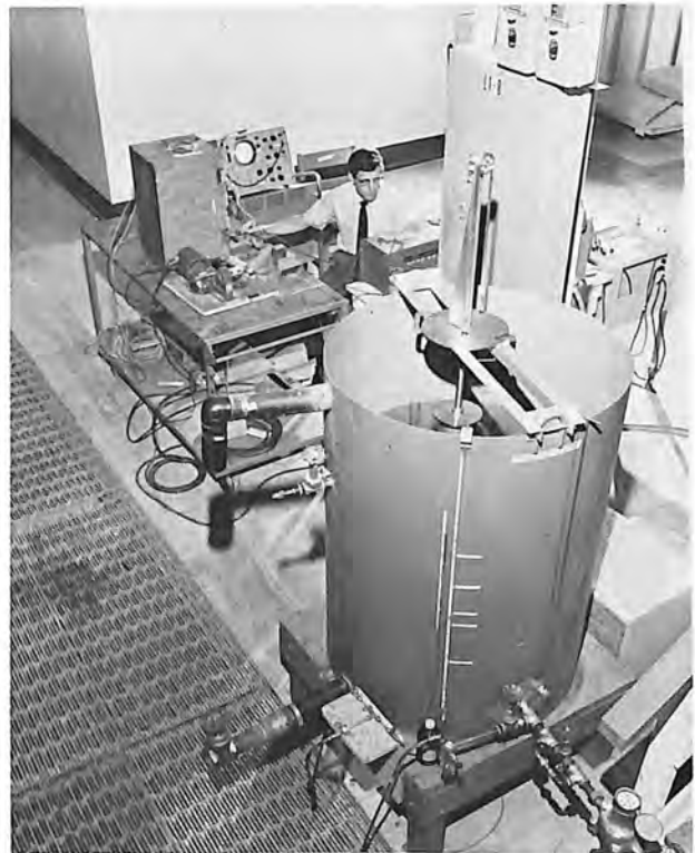
Laboratory studies of the HyFLO water-level sensor and signal generator developed by the Mid-Pacific Region were conducted at the E&R Center.
