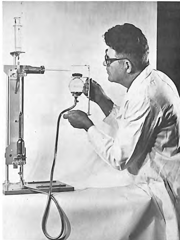
Portable apparatus for determining the dissolved gas content of electrical oils used in transformers and Pirelli-type cables.
