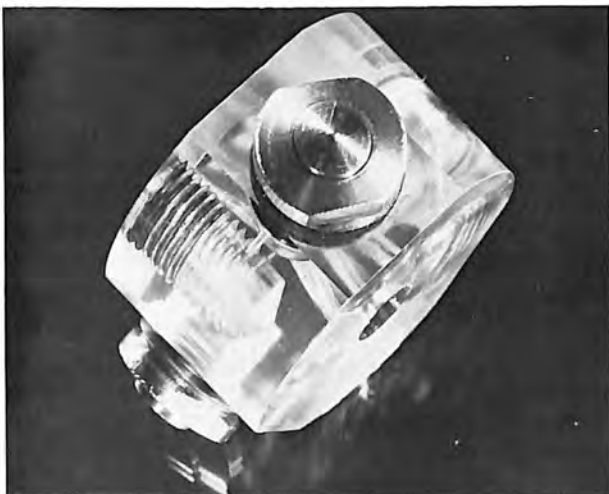
Measuring component for a three-directional borehole gauge.
