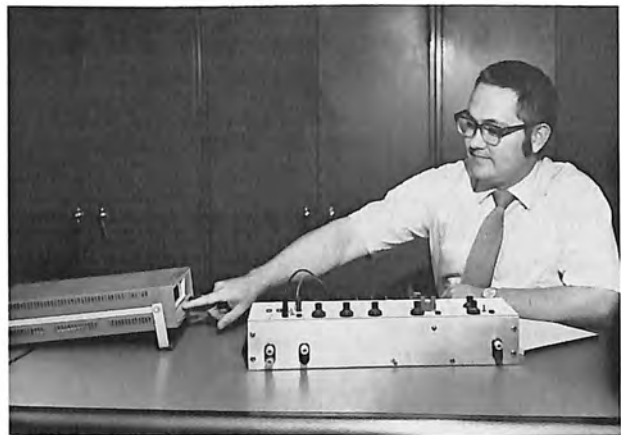
A versatile power system stabilizer was designed and assembled in the laboratory for use in simulation studies and for demonstrating alinement procedures.
