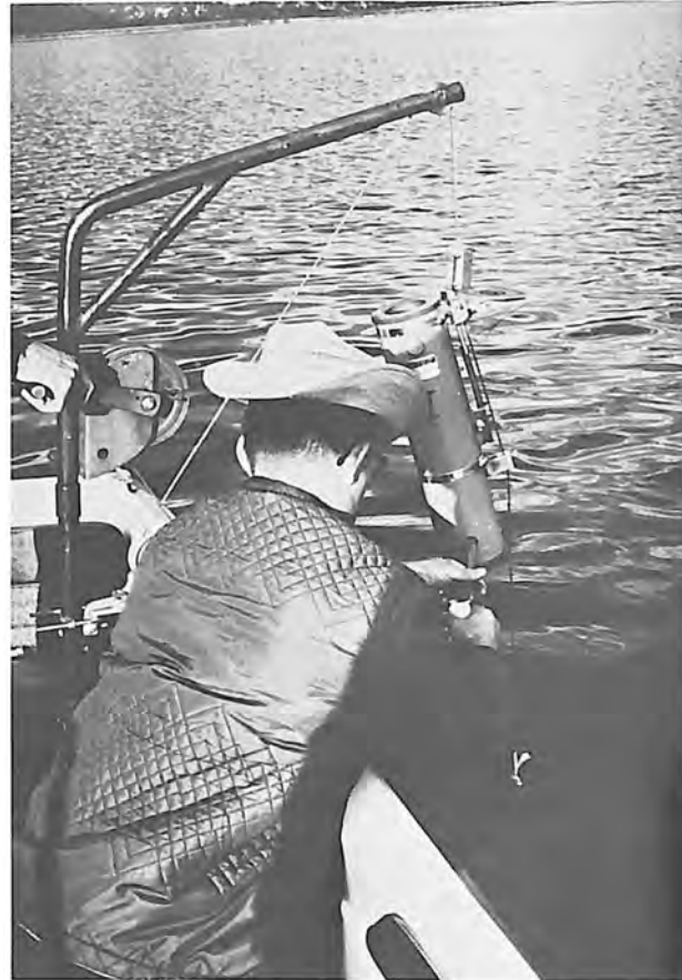
Collecting water samples for dissolved oxygen analysis at Twin Lakes Reservoir.
