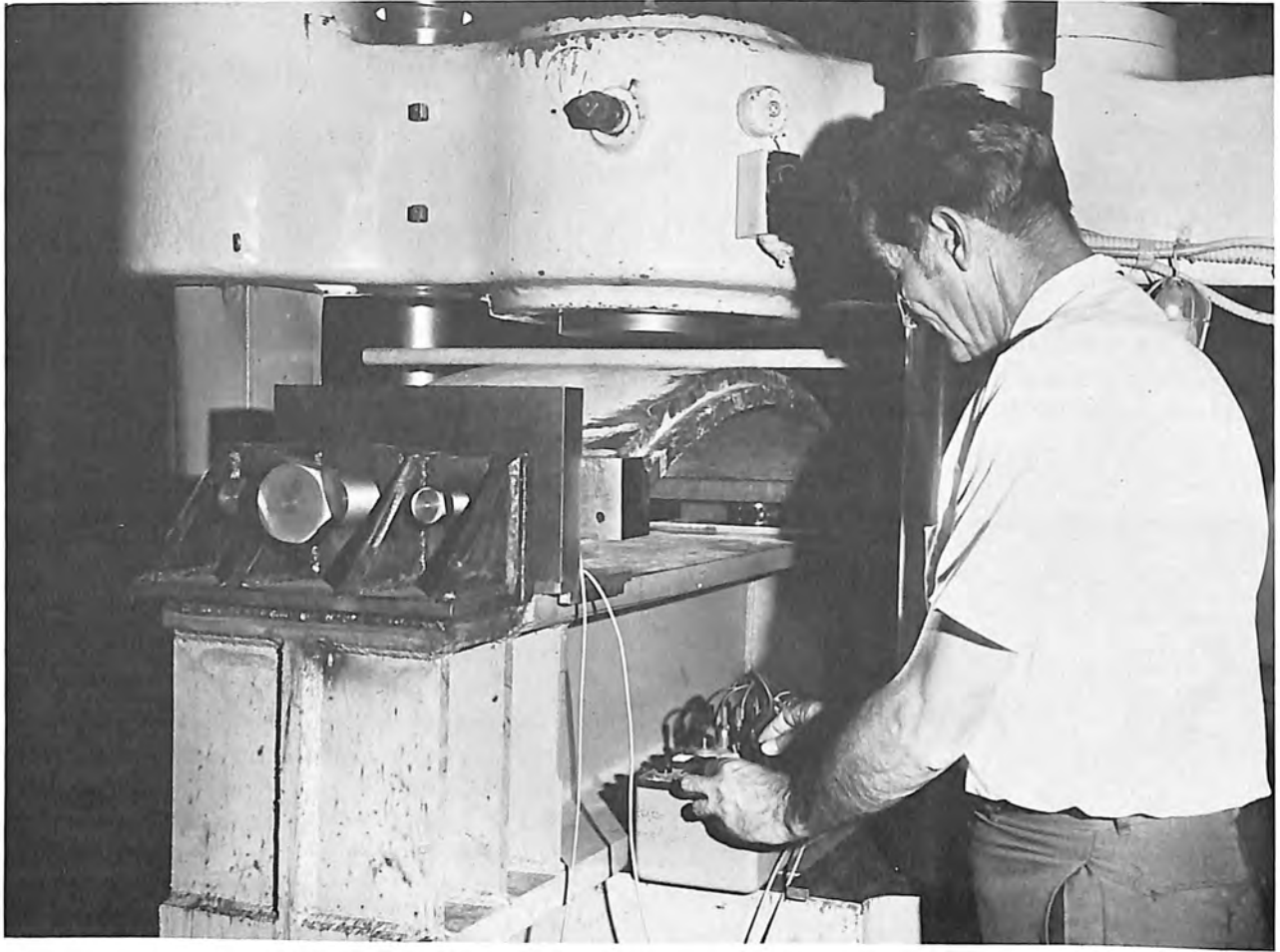
Testing a single precast polymer concrete tunnel support and lining system.
