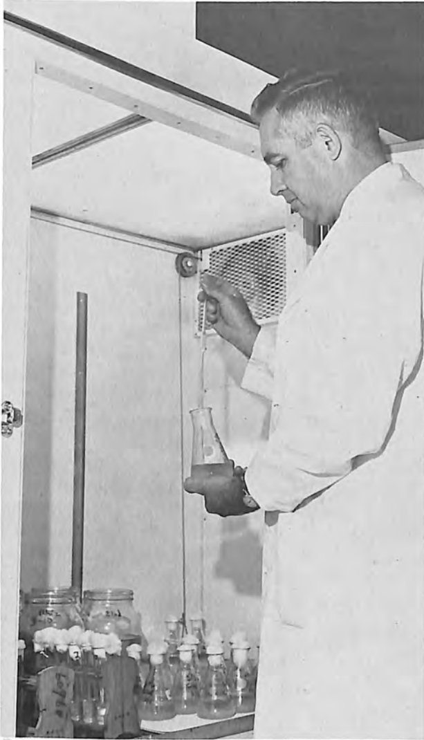
Environmental growth chamber used to culture filamentous green algae utilized in algaecidal studies.
