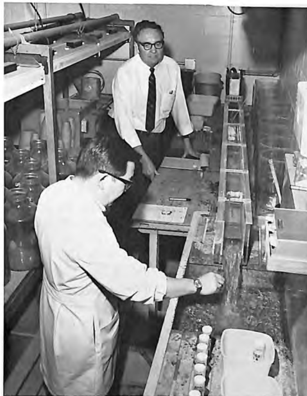
A weed control process using copper sulfate crystals measures the rate at which crystals dissolve at different water temperatures and flow velocities.
