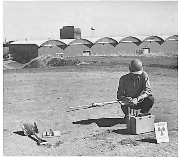
Measurement of soil moisture and density with a nuclear-type gauge.
