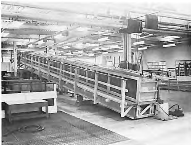
Sloping 60-foot-long flume for pipe drainage tests.
