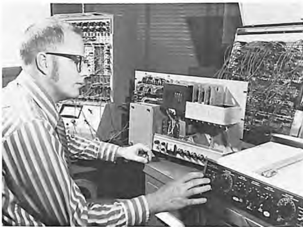
Calibration and operational check of final version of electric governor conversion package by analog simulation of the machine and power system.
