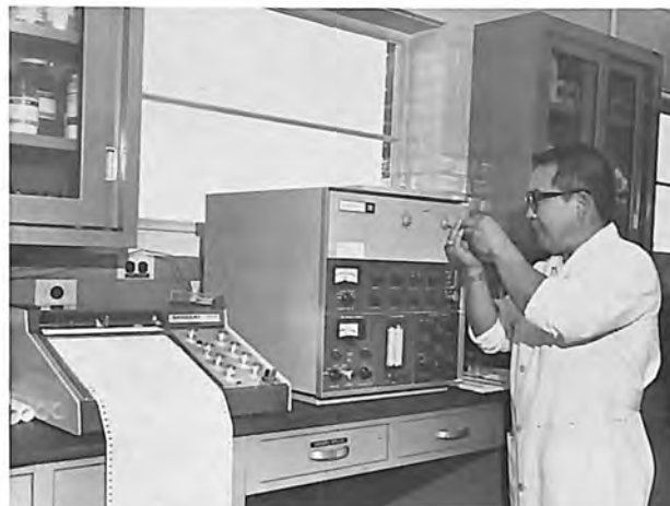
Determining arsenic content of water collected downstream in several canals after ditchbank treatment.
