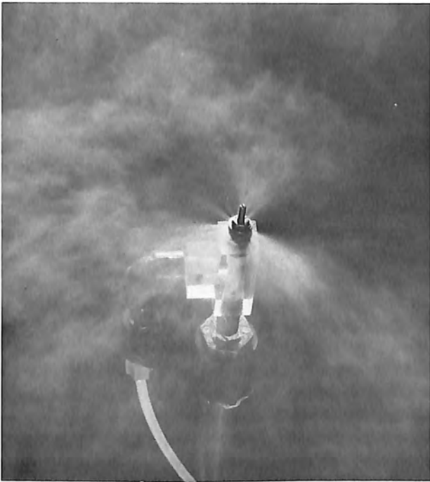
Spray issuing from a commercial "Sonicore" nozzle, which was investigated for seeding warm clouds with hygroscopic solutions.
