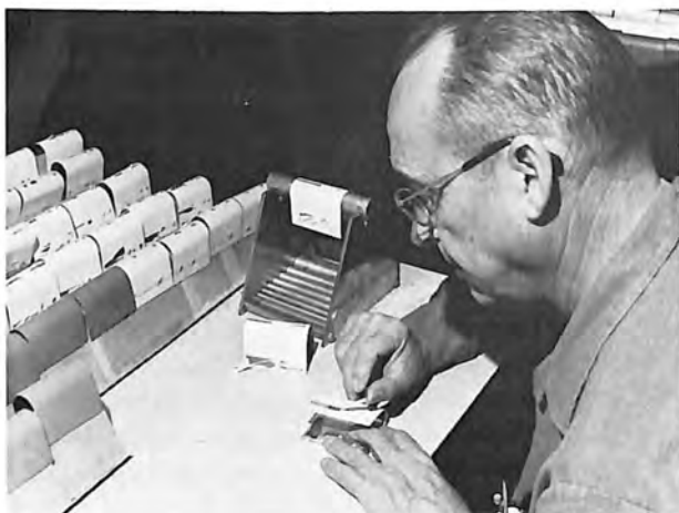
The bond of coatings applied to small panels show how well metal conditioners enhance coating adhesion to nonferrous metals.
