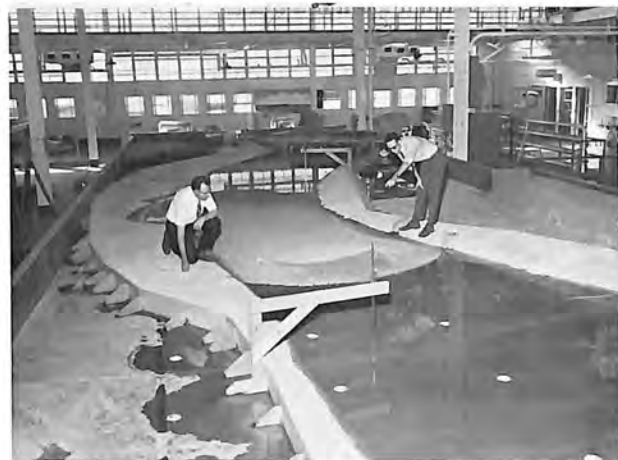
Floating plastic chips simulate an ice jam in a 1:24 scale model of an ice control structure on the North Platte River near Casper, Wyo.
