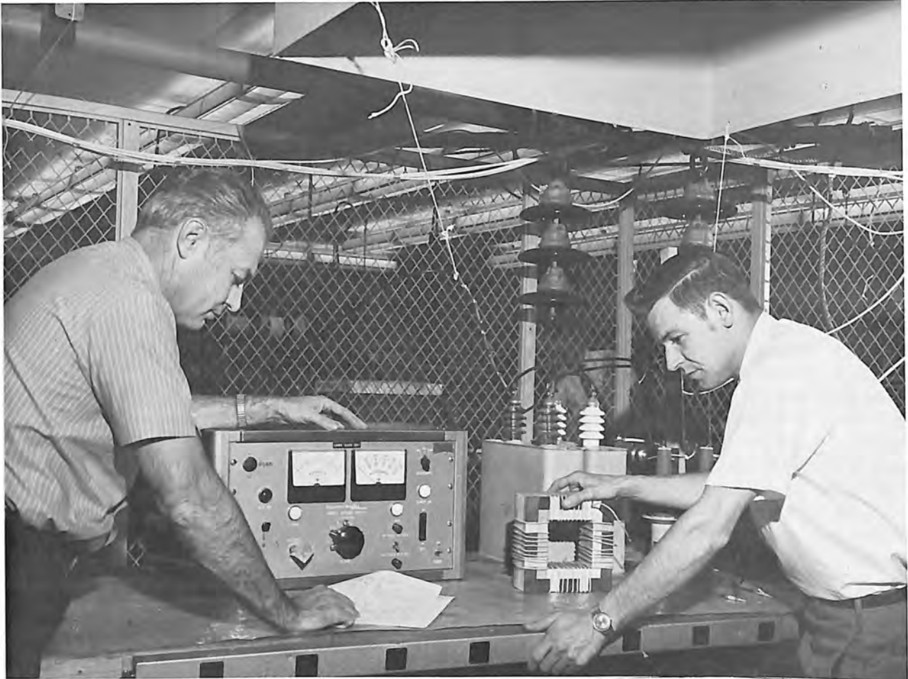
Substation switching transients were simulated in the laboratory high-voltage cage by an impulse generator feeding a simulated high-voltage bus.
