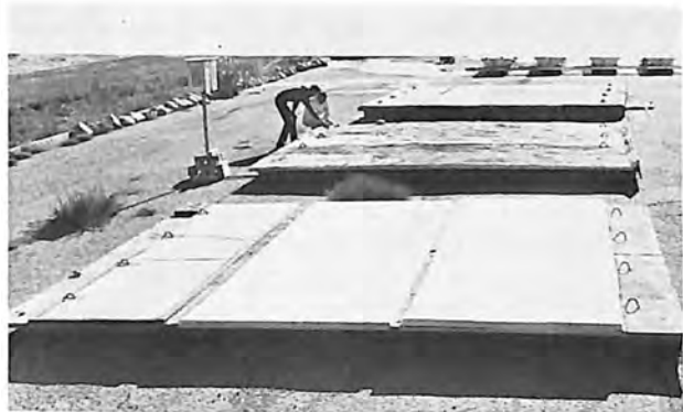
Outdoor exposure test areas are used for investigating various roofing systems.
