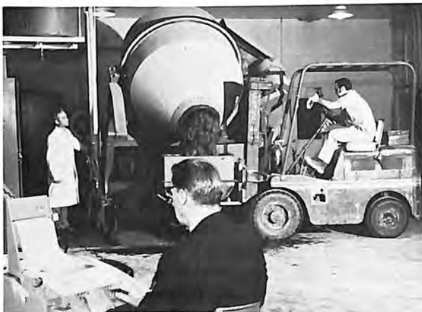
Mix designs for best economy and desired performance are made in the laboratory using project aggregate, cements, and admixtures.
