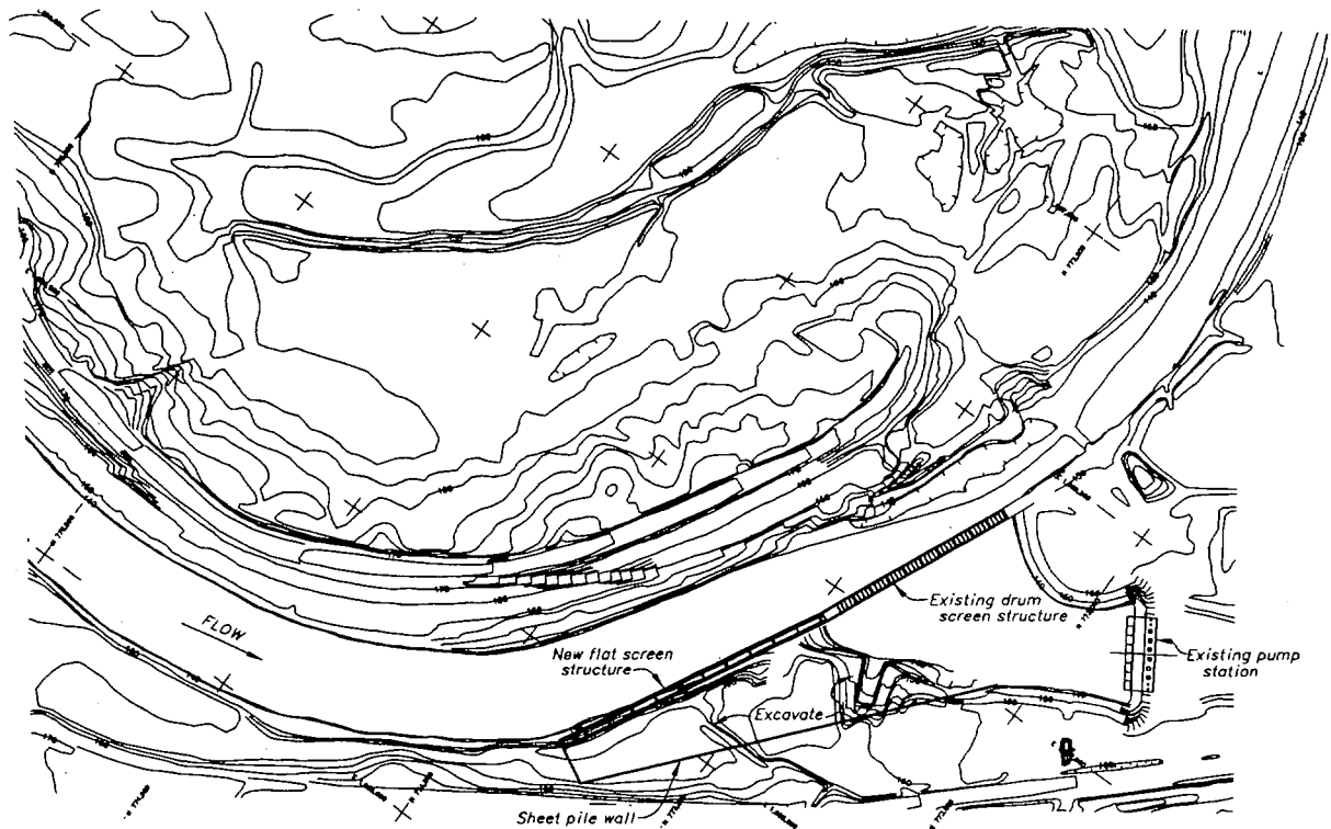
Figure 3. - Conceptual layout: plan view of proposed D alternative.
