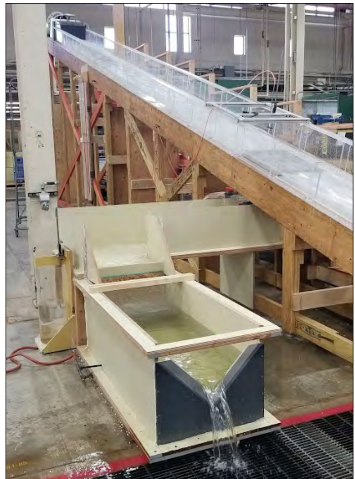
Figure 3 Hydraulic Jacking Research Flume Showing the Jet Box (top), Spillway Joint (right foreground), and Receiving Channel and V-Notch Weir (foreground)
