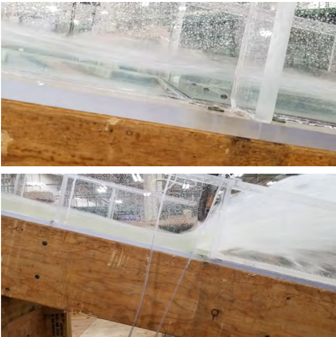
Figure 7 Flow Attached to the Flume Floor as It Passes Over a Small Offset (top), and a Free Jet Detached From the Floor by a Large Offset (bottom)
