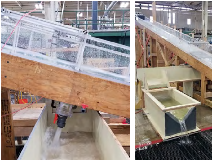
Figure 6 Valves Regulate the Backpressure and Flow Out of the Chamber Below the Joint, and the Joint Flow Is Measured Through a V-Notch Weir
