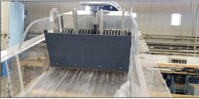
Figure 4 A Jet Box Regulates the Depth and Velocity of Incoming Flow
