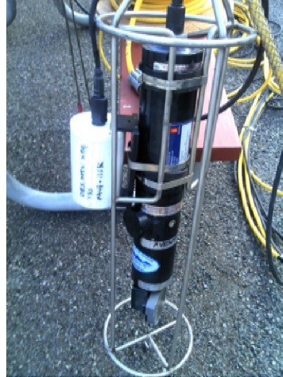
Figure 3. Photograph of scanning sonar and MRU (white cylinder).
