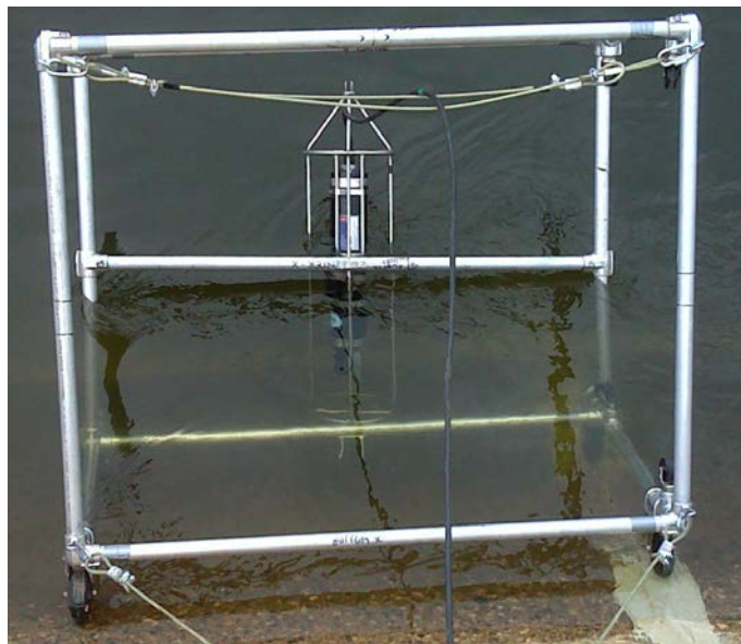
Figure 4. Photograph of cage with sonar mounted so the transducer was oriented perpendicular to image the concrete surface (Note: this photo was not taken at Buffalo Bill Dam).
