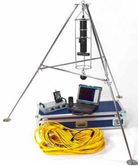
Figure 3. Photograph of a KML MS1000 Scanning Sonar System similar to the one used for this project. (Photo courtesy of Kongsberg-Mesotech Ltd)
