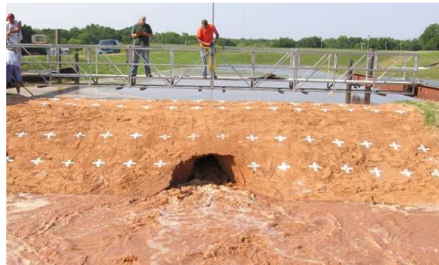
Figure 1. — ARS piping test P1, 9 minutes after initiation of piping failure.
