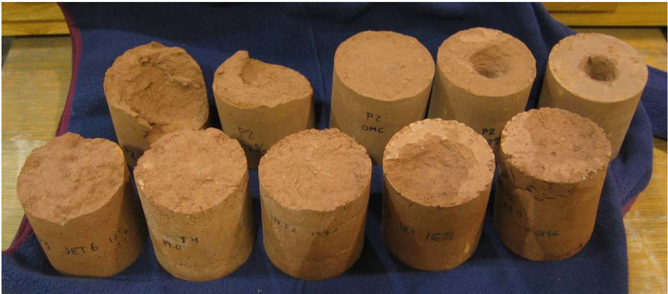
Figure 11. — Changes in erosion mode for JET specimens of soils P2 (back) and P3 (front) as a function of changing compaction moisture content. Driest specimens at compaction are on the left and wettest specimens are on the right.
