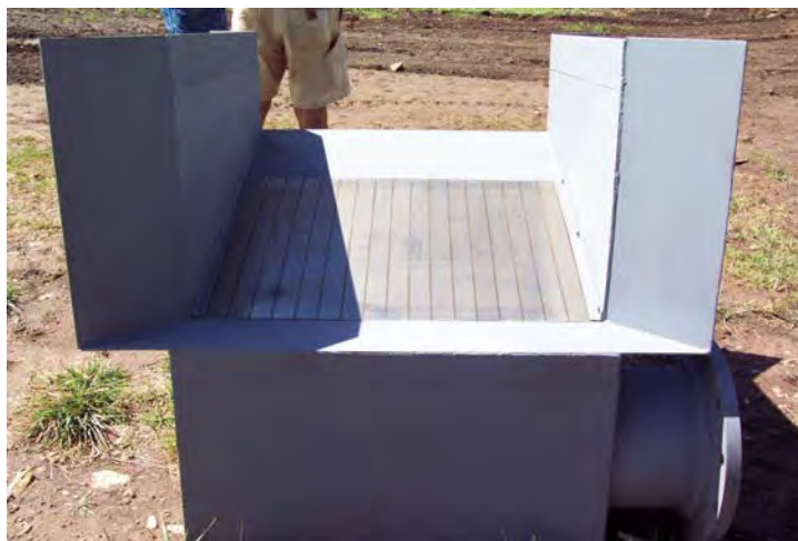
Figure 12. — Modular Coanda-effect screen structure. Flow is toward the reader. Screened flow exits to the right through the flanged pipe connection.
