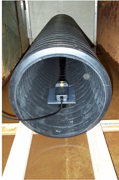
Figure 4. Looking upstream at the SW in plastic pipe section. The SW was positioned 2.3 m downstream from the pipe entrance.
