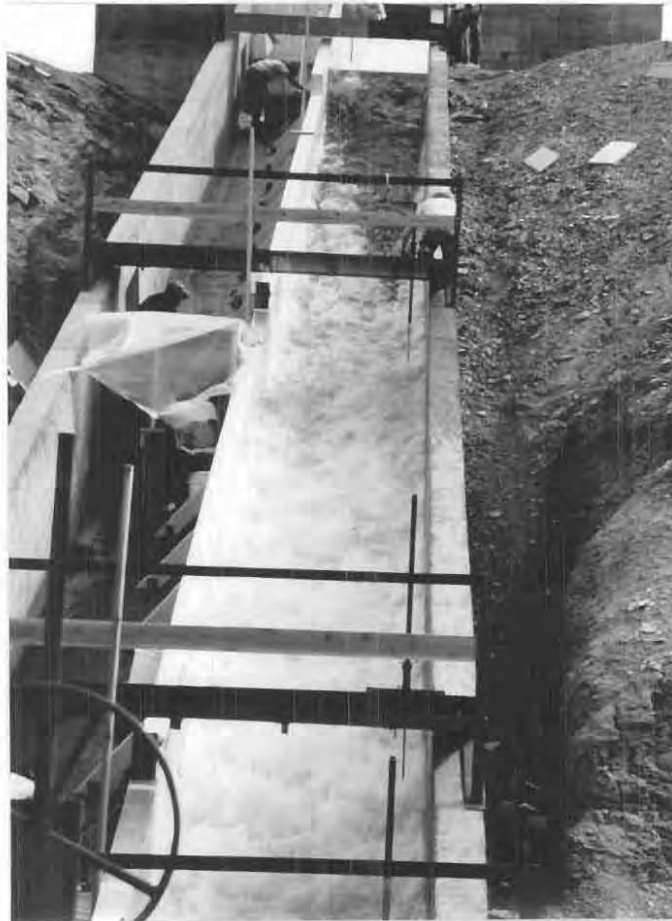
Figure 1. - Large-scale, 50-ft-high, dam overtopping test facility, q = 32 \text{ ft}^3/\text{s}/\text{ft} .
