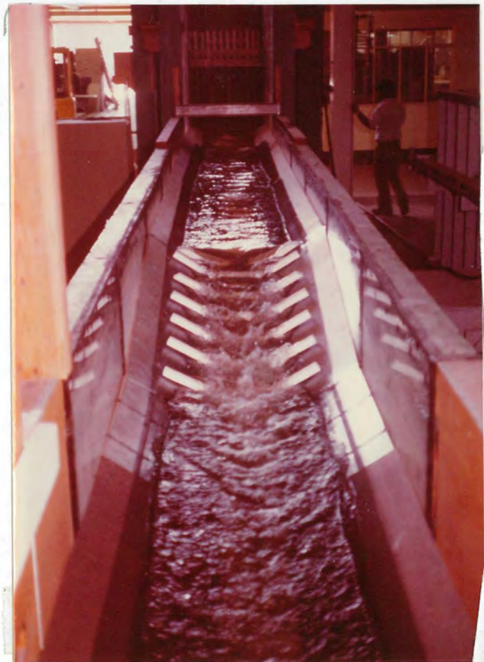
Figure 16 - Flow conditions at 8.33 m 3 /s (294 ft 3 /s).
