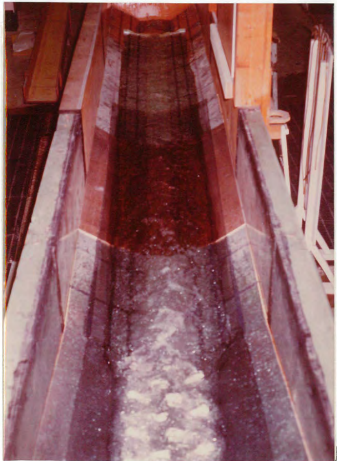
Figure 8 - Flow of 8.33 \text{ m}^3/\text{s} ( 294 \text{ ft}^3/\text{s} ) with lower con- trol notch in place.
