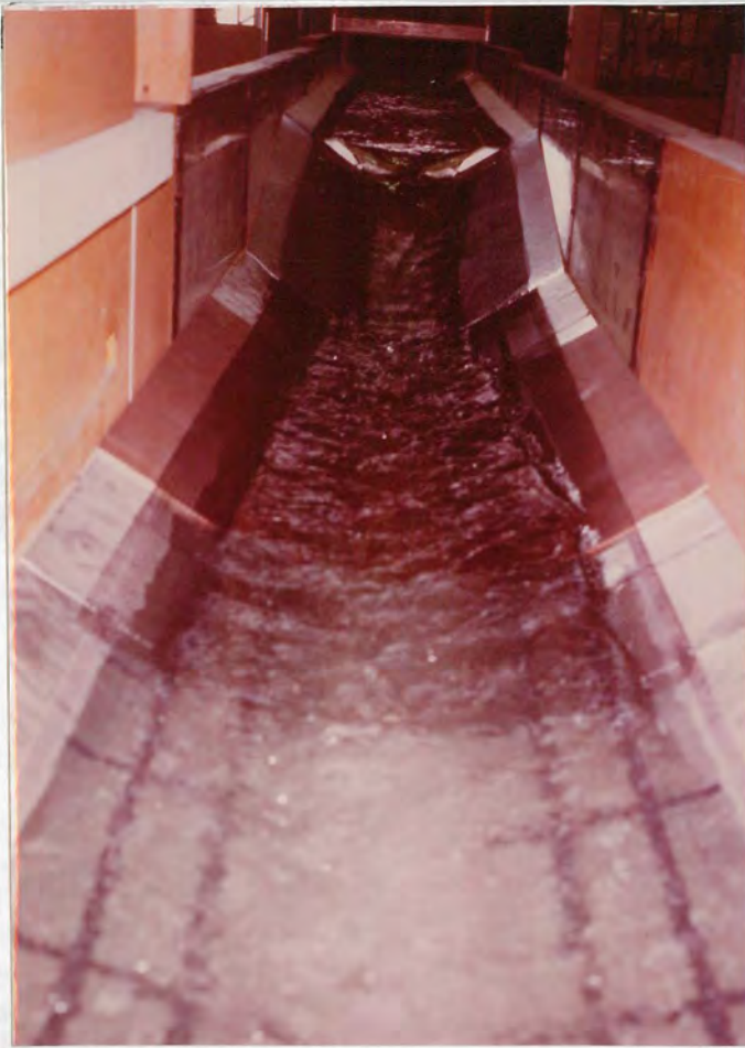
Figure 3 - View of downstream water surface with lower control notch in place.
