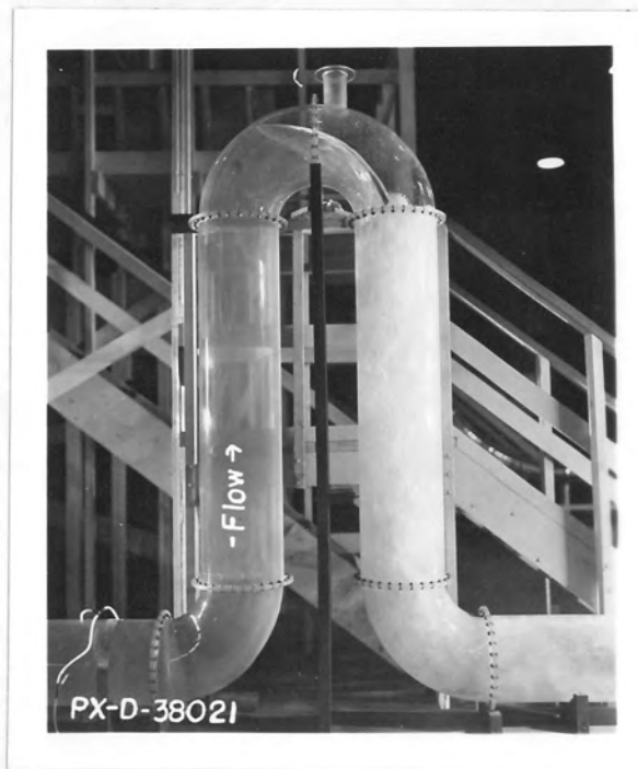
FIGURE 3. TYPICAL CHECK TOWER--CANADIAN RIVER AQUEDUCT, TEXAS
