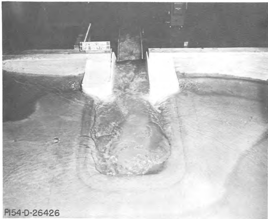
B. Closeup of flow in Fontenelle Dam spillway. U-shape spillway showing submergence and flow concentration on right side. Discharge = 20,000 cfs.
