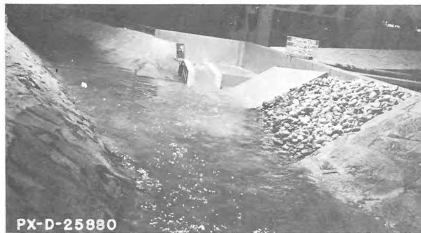
C. Stilling basin performance and riverflow conditions for a diversion flow of 20,000 cfs.
