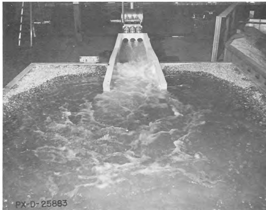
A. Flow appearance with three conduits operating at 19,000 second-feet maximum discharge.
