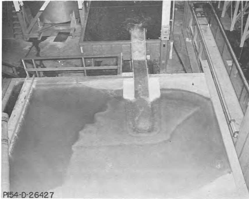
A. Overall view of Fontenelle Dam spillway 1:30 scale model. Discharge = 20,000 cfs.
