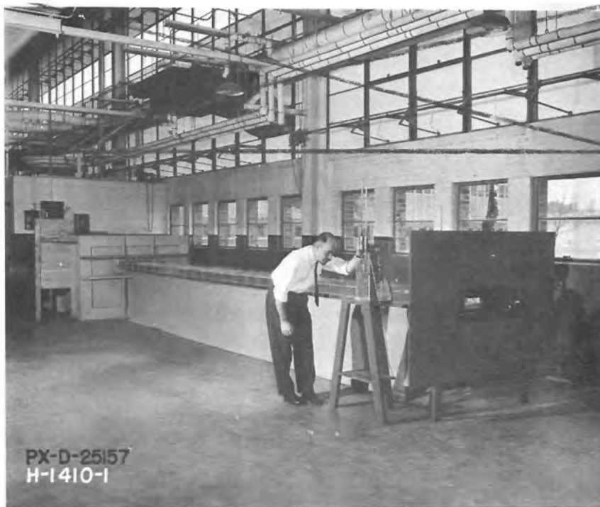
Figure 10 Air test facility for study of boundary surface resistance coefficients.
