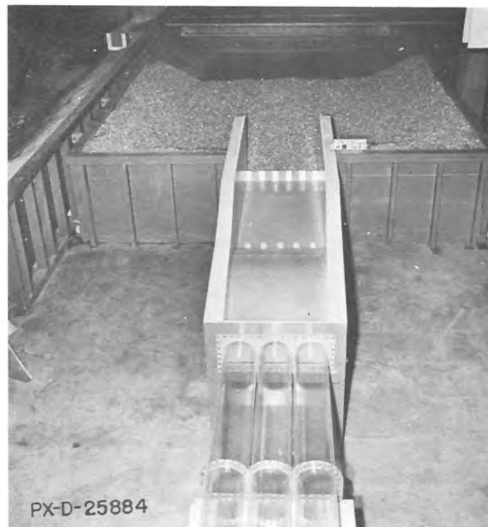
B. Riprap protection in channel below stilling basin.
