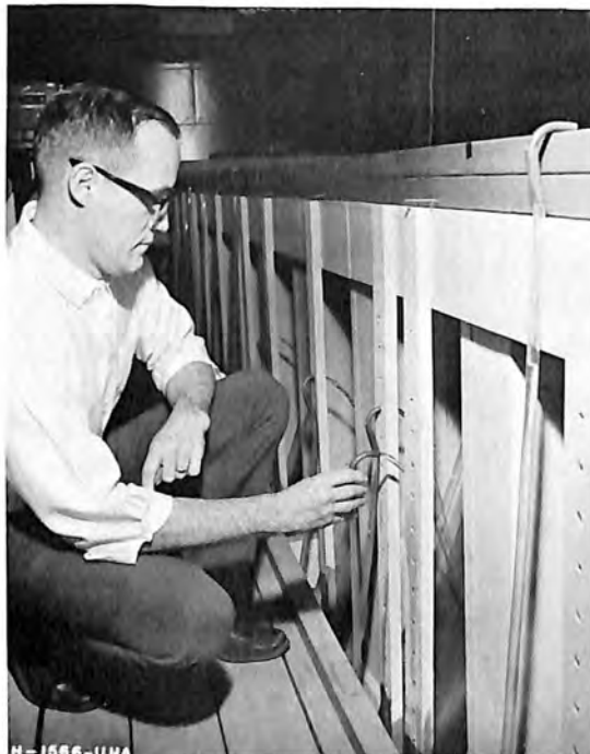
B. Adjusting outflow tubes to set a seepage rate. Photo PX-D-60405
