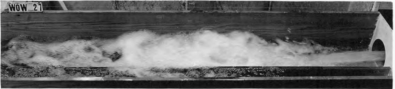
A. ONE VALVE 14.9% OPEN; CENTERLINE EL. 4258; DISCHARGE 381 S.F.; T.W. EL. 4260.3.
