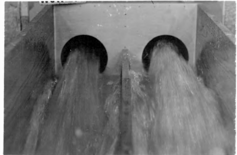
D. RECOMMENDED DISCHARGE GUIDE VANE; 1975 SECOND-FEET PER VALVE; LEFT JET AERATED.
