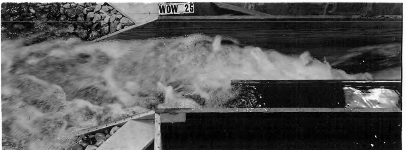
C. RECOMMENDED DESIGN; RIGHT VALVE 1975 SECOND- FEET.
