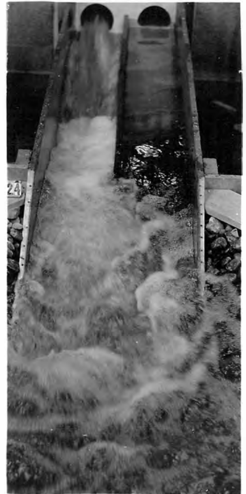
B. RECOMMENDED DESIGN; RIGHT VALVE 1975 SECOND- FEET.
