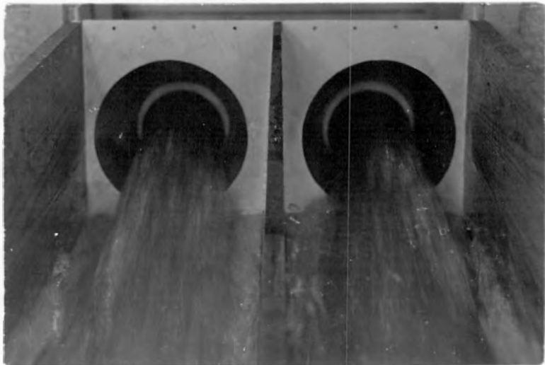
C. ORIGINAL DISCHARGE GUIDE VANE; 1975 SECOND-FEET PER VALVE.
