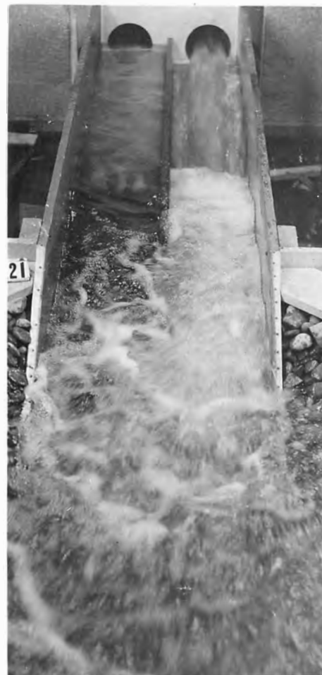
B. RECOMMENDED DESIGN; LEFT VALVE 1975 SECOND- FEET.
