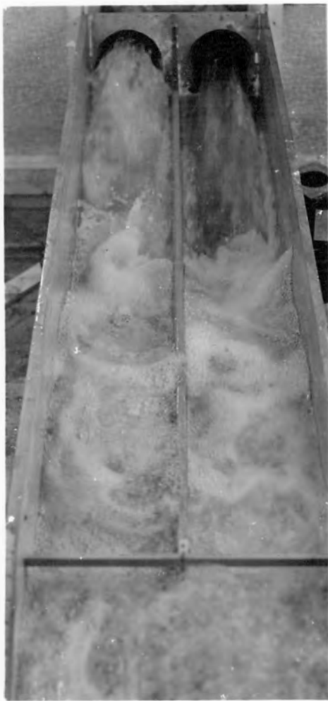
A. 1975 SECOND-FEET PER VALVE; RIGHT JET AERATED; LEFT JET SOLID.
