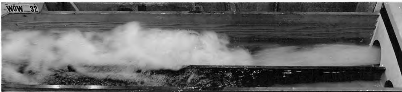
A. ONE VALVE 32.6% OPEN; CENTERLINE EL. 4258; DISCHARGE 887 S.F.; T.W. EL. 4261.8.
