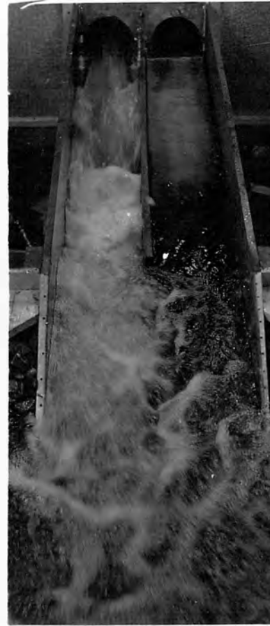
C. 20 FEET SHORTER AND 4 FEET LOWER DIVIDING WALL; 1975 SECOND-FOOT.
