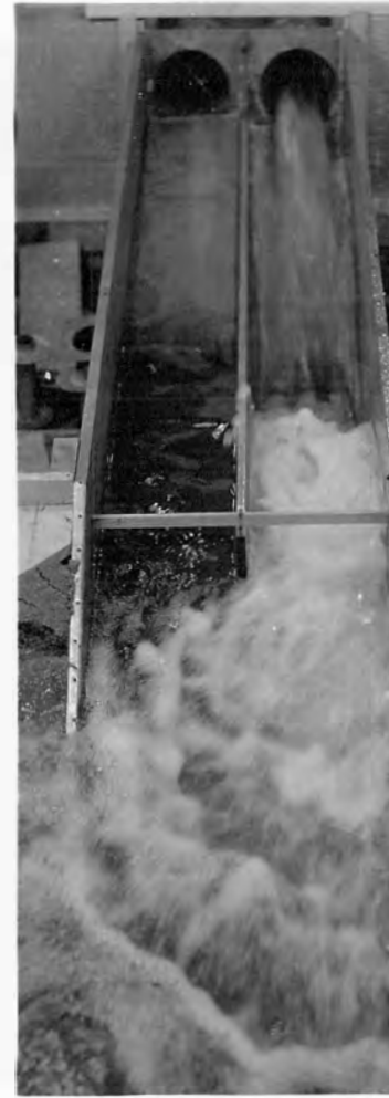
D. 1975 SECOND-FEET; FLARED CHUTE WALLS; FLOOR EL. 4247.
