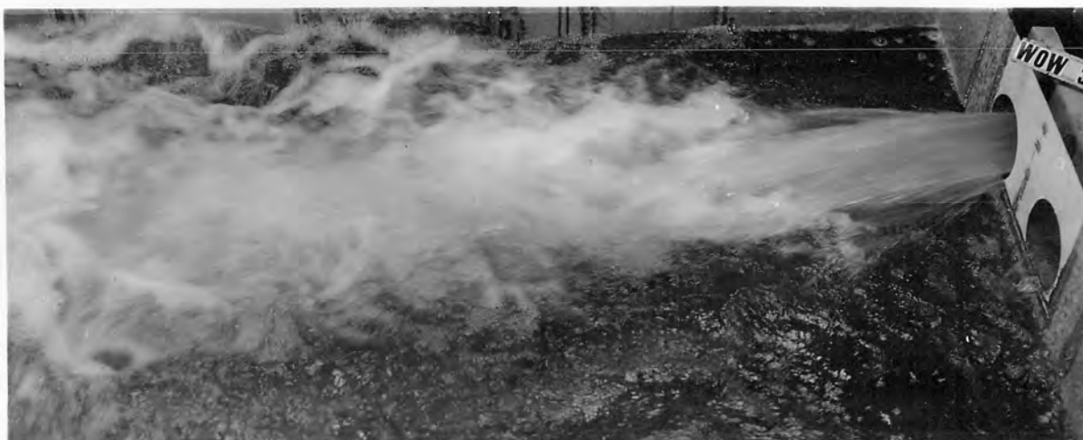
C. 1975 SECOND-FEET; VALVE CENTERLINE EL. 4268; TAILWATER EL. 4264.4.
