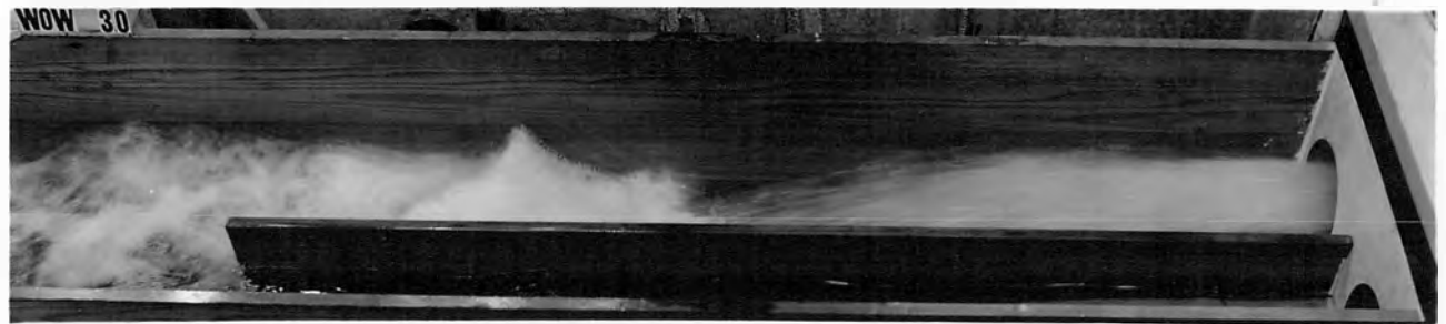
D. ONE VALVE 32.6% OPEN; CENTERLINE EL. 4263; DISCHARGE 887 S.F.; T.W. EL. 4261.8.
