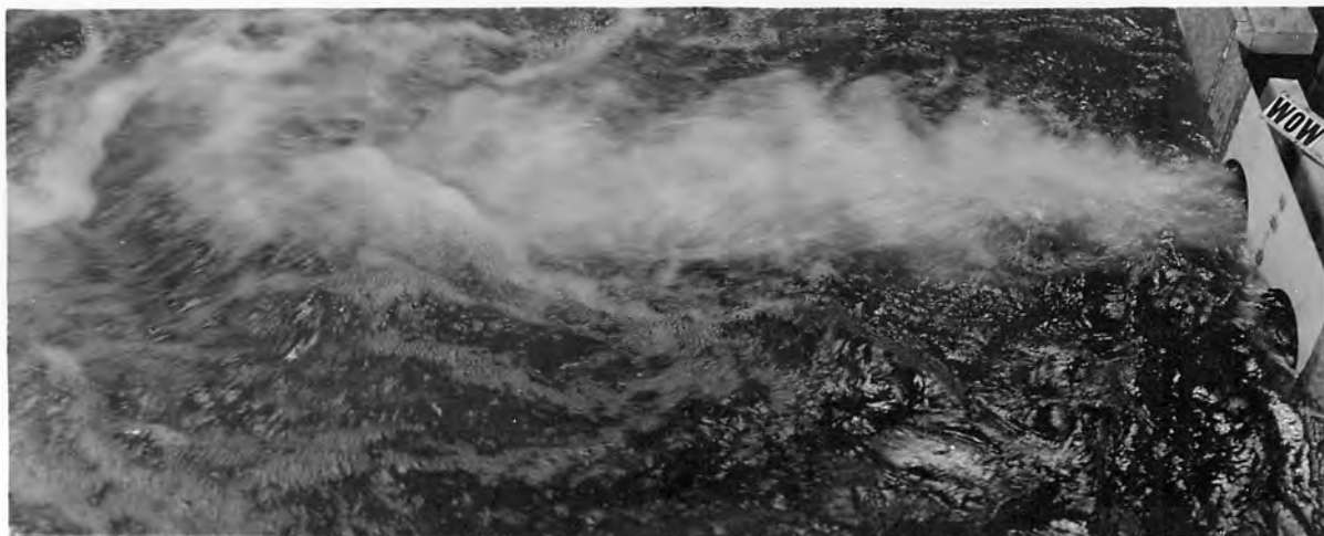
A. 1975 SECOND-FEET; VALVE CENTERLINE EL. 4260; TAILWATER EL. 4264.4.
