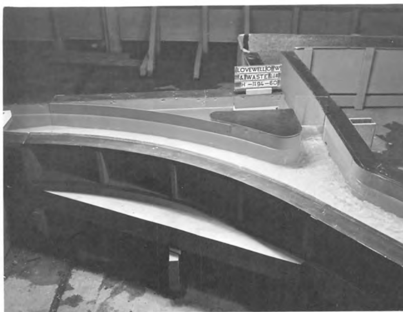
A. Original Wasteway Entrance Closed by Curved Wall and New Entrance Provided Downstream.
