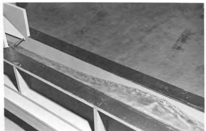
Standing waves move to Station 3+58 when gate is closed 7%. At greater closures the wave disappears.
