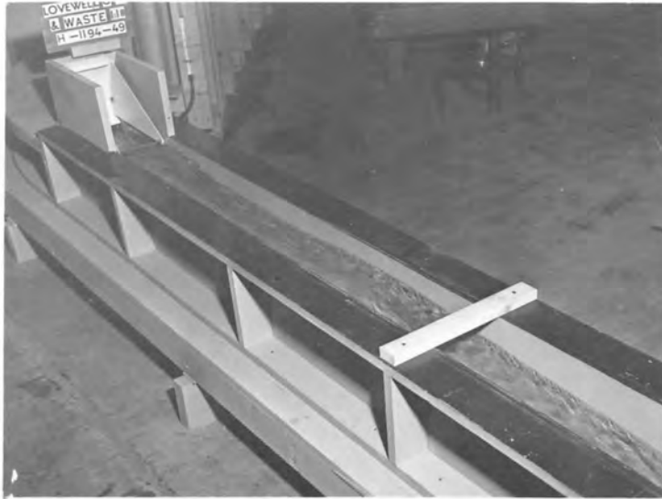
A. Water Passage below Control Gate.
