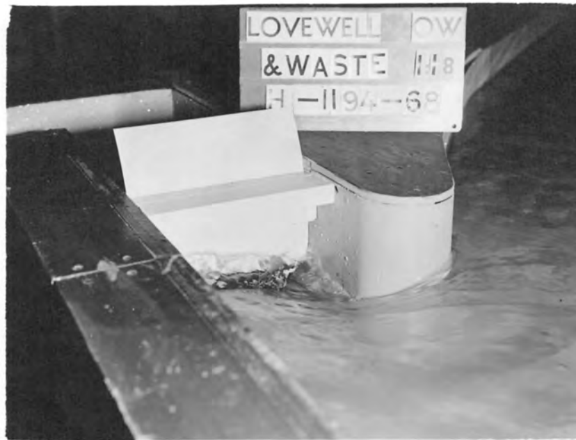
A. Gate Controlling the Flow with Water Surface Elevation at Canal Entrance--1570.50.
