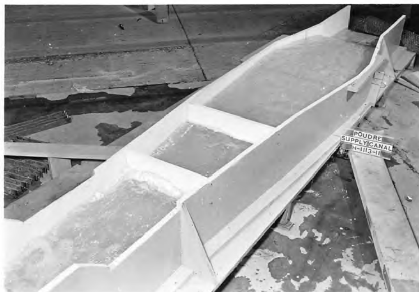
C. Smooth flow in measuring flume at 1250 cfs.
