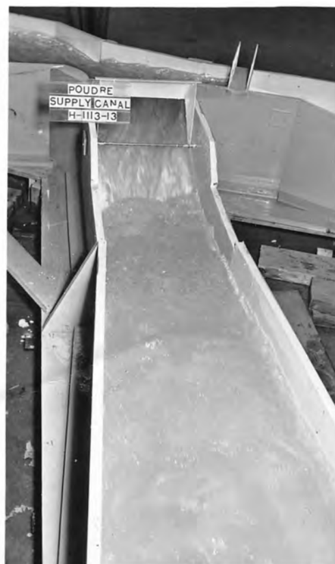
B. Appearance in stilling basin at 1250 cfs.
