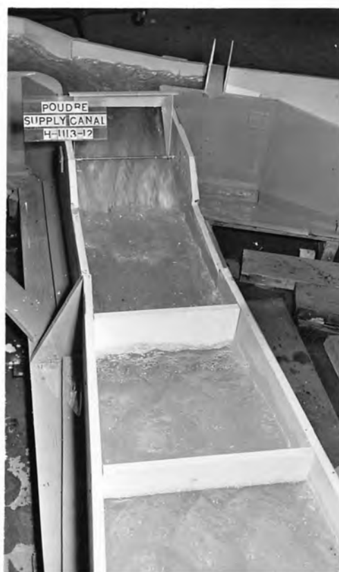
B. Stilling basin performance at 1250 cfs.
