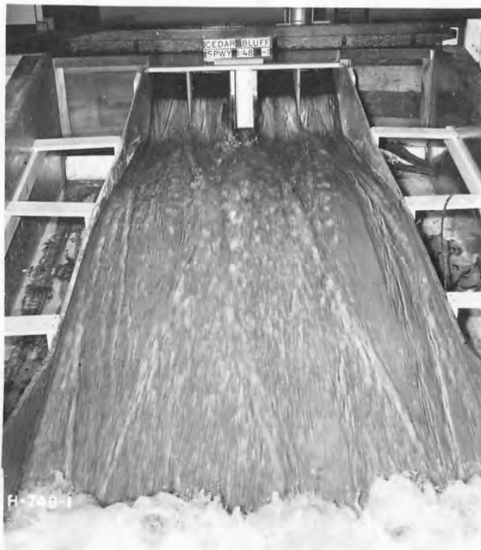
A. Piers in place, 116 feet crest length Discharge 72,000 second-feet
