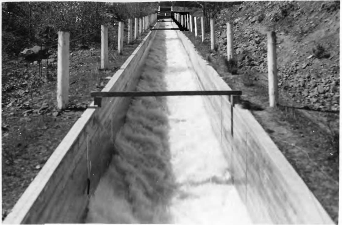
A. FLOW CONDITIONS ON 10^{\circ} - 12' SLOPE. DISCHARGE 777 SECOND-FEET.
