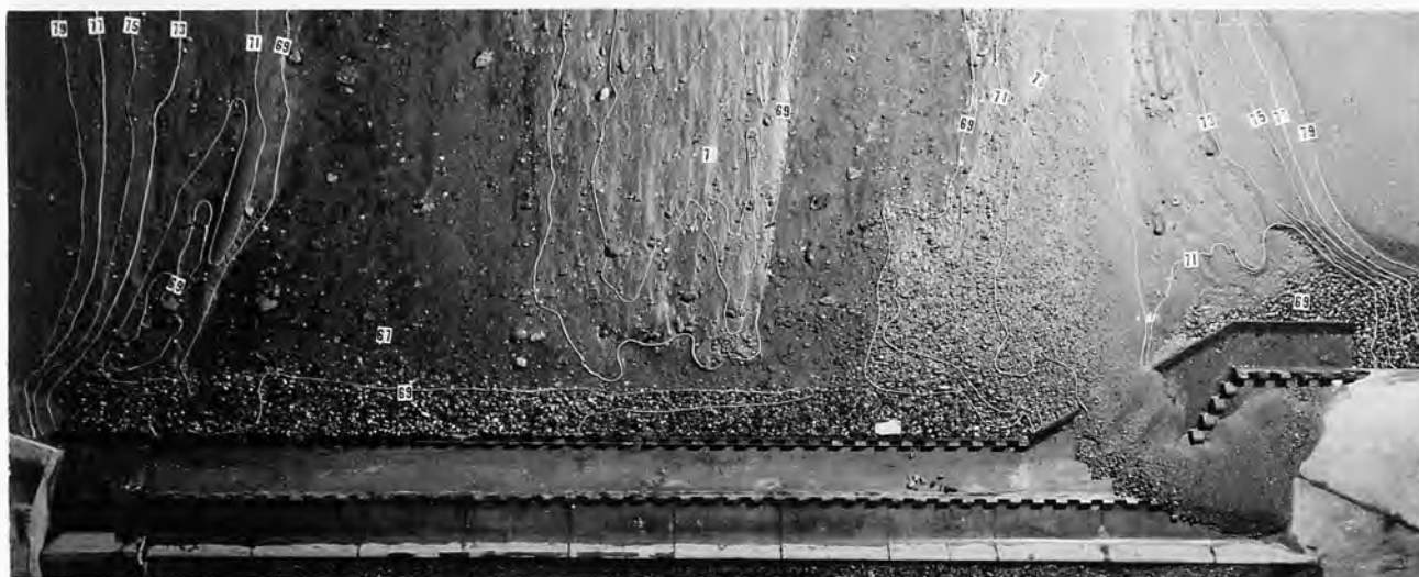
B. RIVER BED AFTER CONSTANT CONDITIONS WERE OBTAINED WITH A FLOW OF 30,000 SECOND-FEET.
