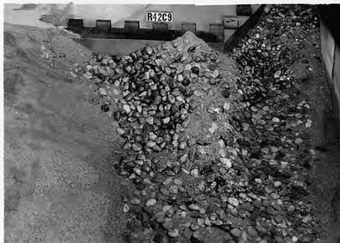
E. SCOUR AT END OF APRON.
