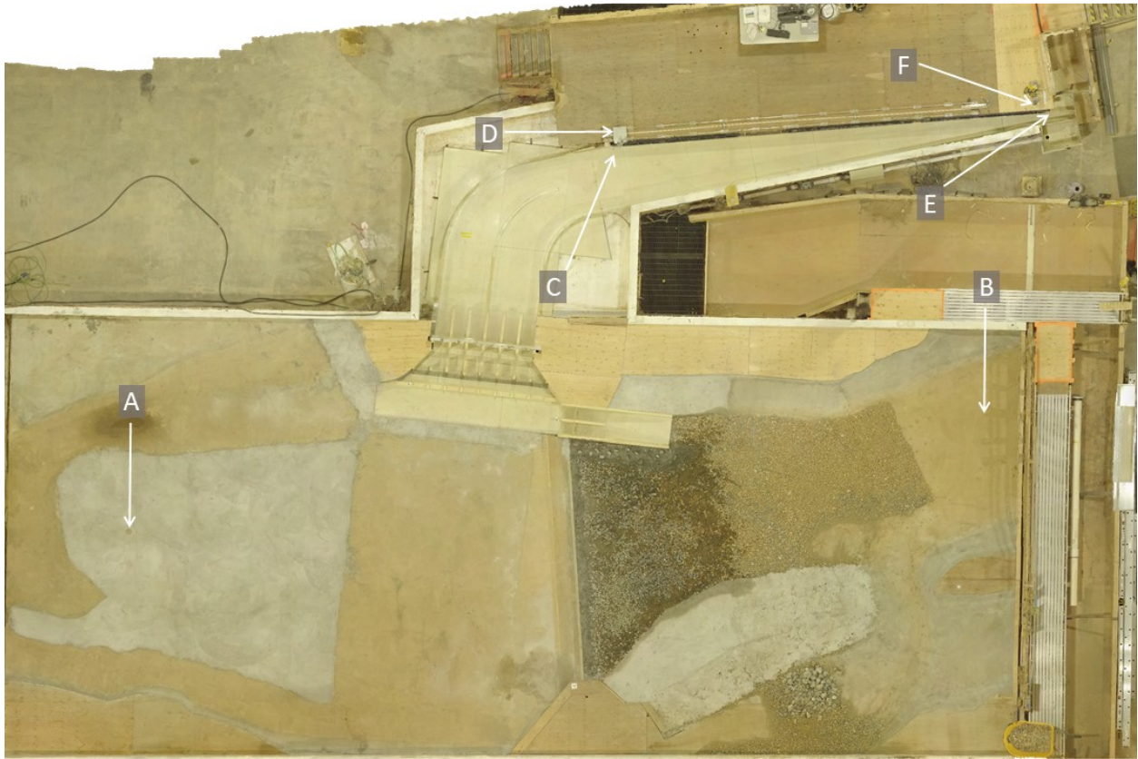
Figure 24. Location of head measurements taken in the St. Mary Diversion Dam model.
