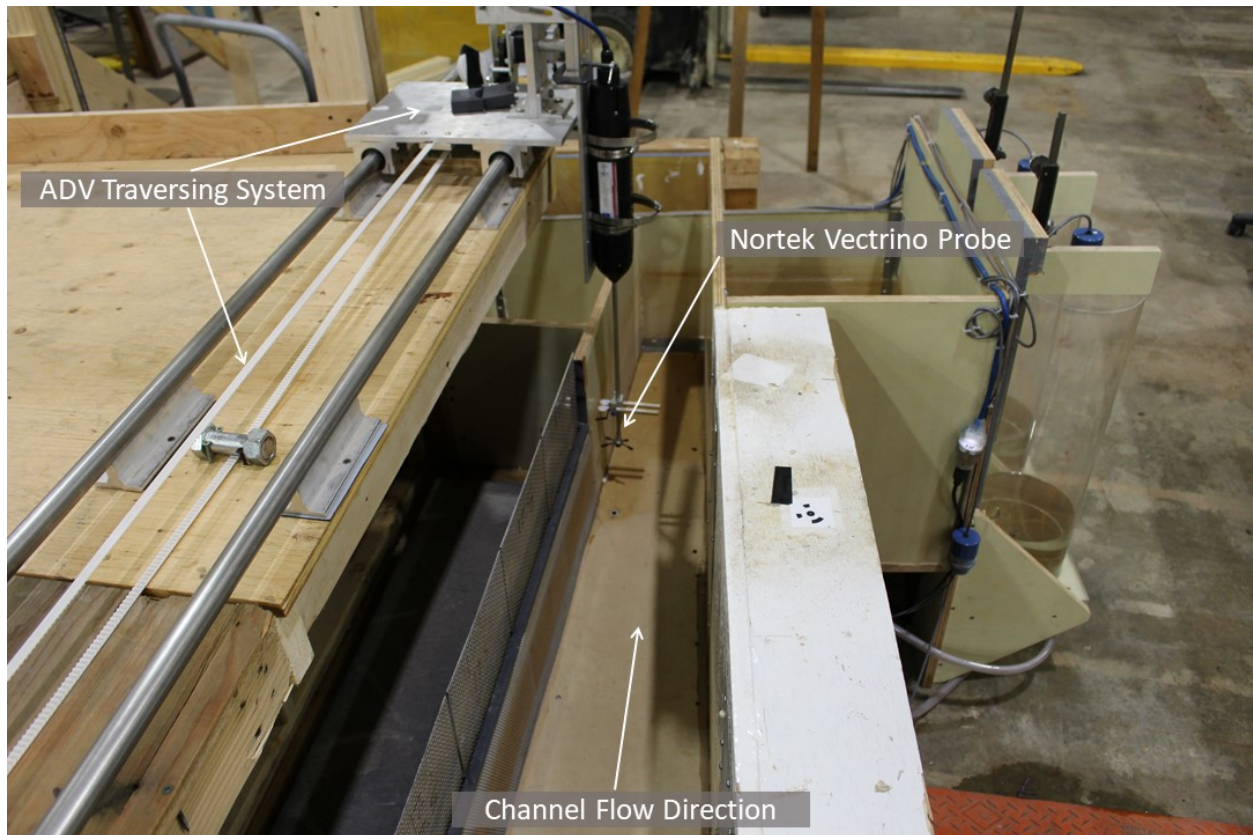
Figure 25. Nortek Vectrino+ 3D velocimeter mounted in the model at 0.50 depth centered at the end of screen number 30.
