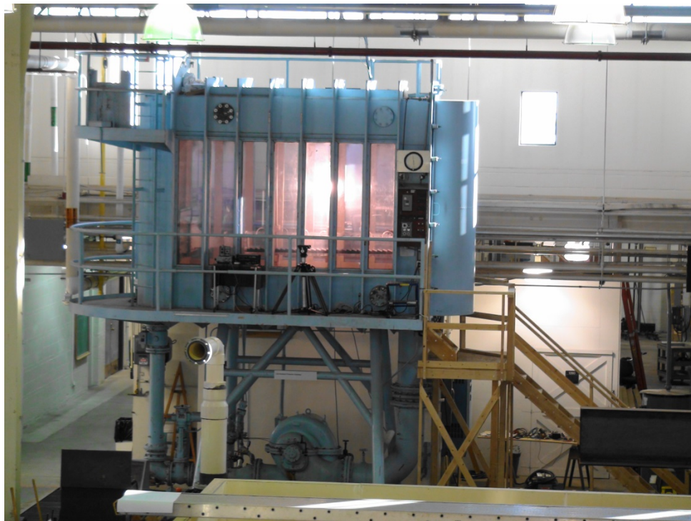
Figure 1: Low Ambient Pressure Chamber, Bureau of Reclamation Hydraulics Laboratory
