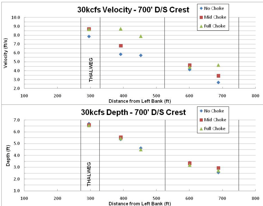
Figure 32 Comparison of velocity and depth data 700 ft downstream of the crest with different choked conditions at 30,000 ft 3 /s; thalweg was not fully choked.
