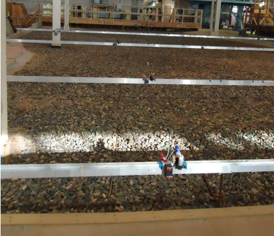
Figure 11. MassaSonic sensors placed next to Nixon meters to record depth and velocity simultaneously at the same location.
