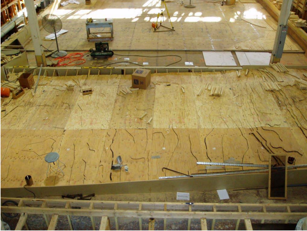
Figure D- 2. Upstream topography meeting diversion weir.
