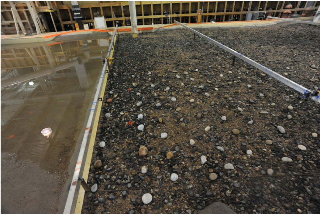
Figure 16. Example of a boulder field tested on the model rock ramp.
