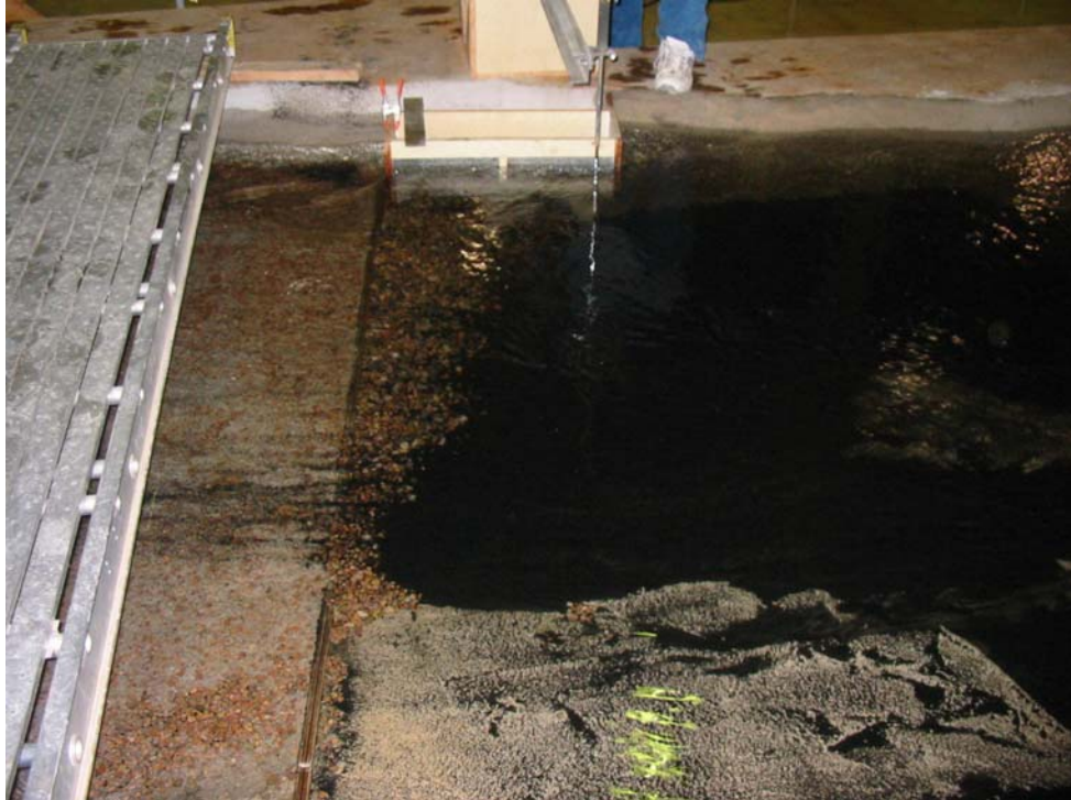
Photograph 21.—View during descending flow following the 14,400 ft 3 /s peak flow. Flow shown is 7,000 ft 3 /s.
