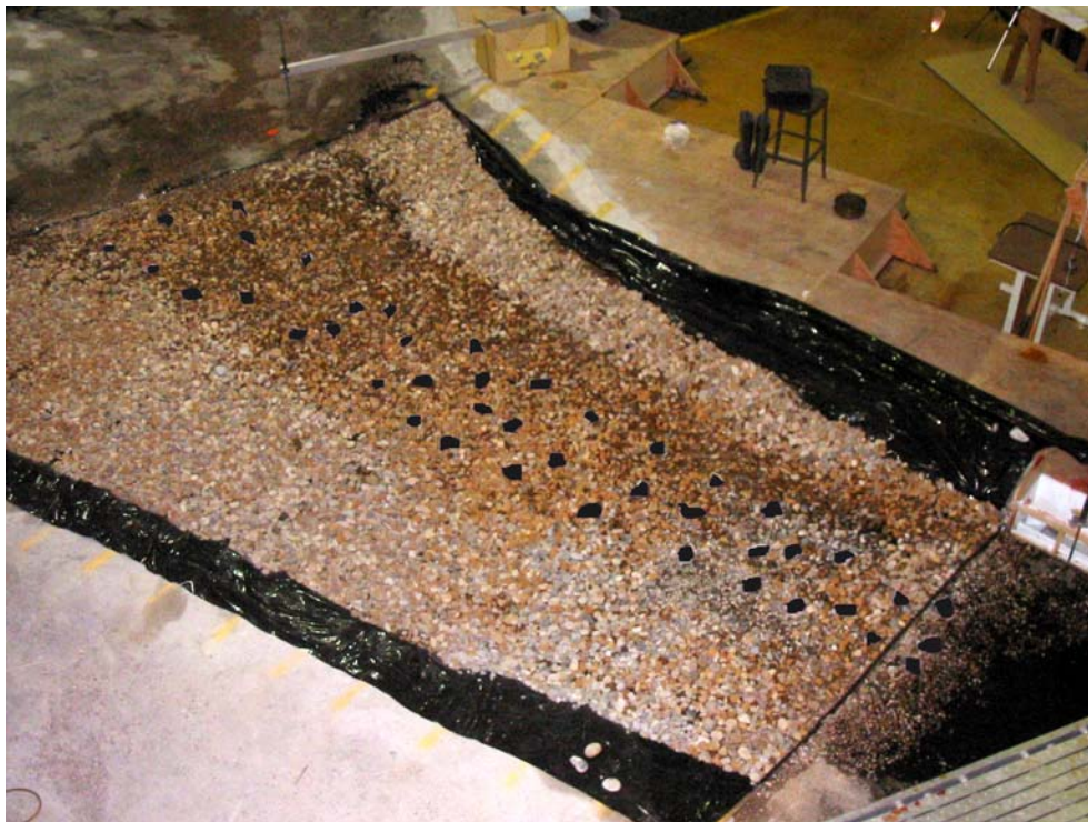
Photograph 24.—View looking downstream of rock ramp with mid-channel boulders shown in black.
