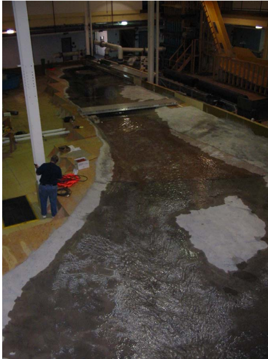
Photograph 6.—View of model during a steady-state flow of 4,000 ft 3 /s.
