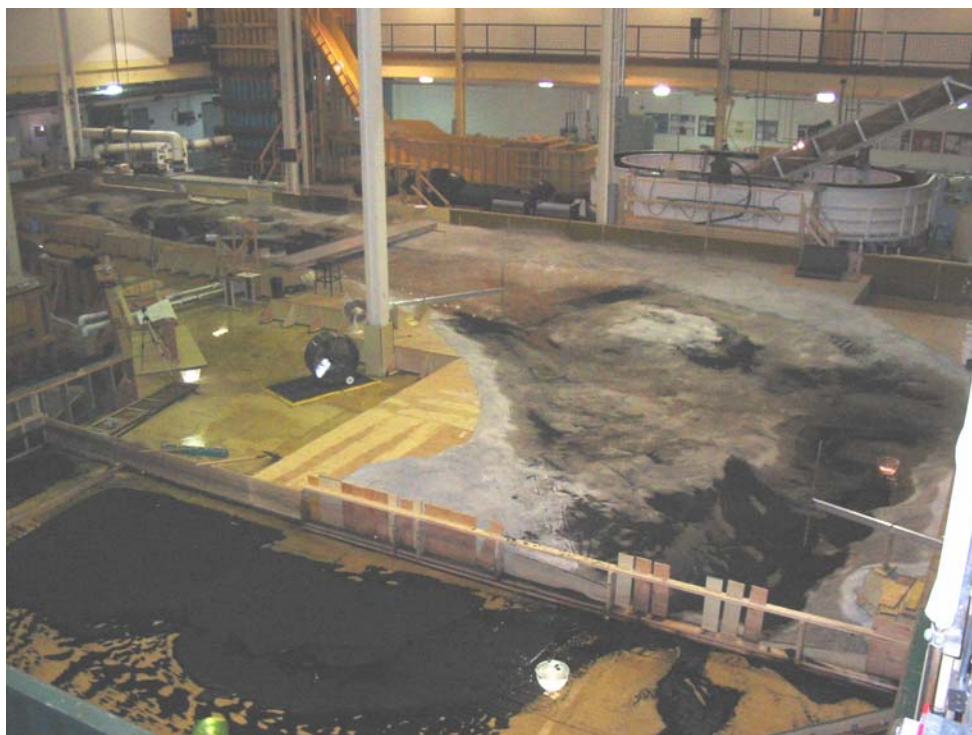
Photograph 4.—View looking upstream of Elwha surface-water intake model.
