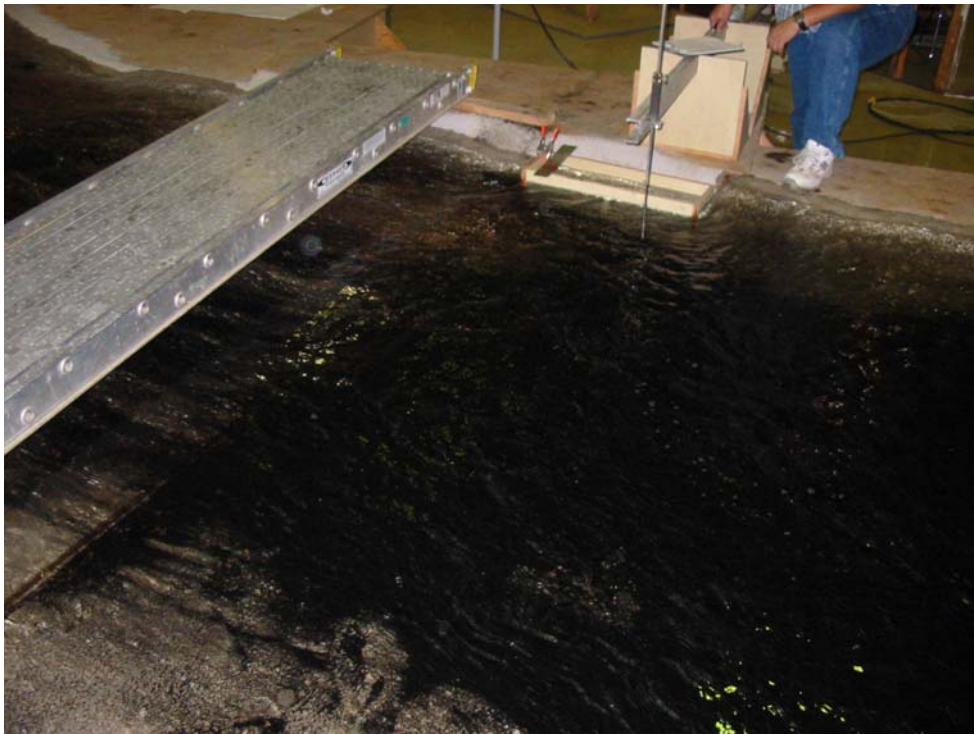
Photograph 20.—View of 14,400 ft 3 /s flow transporting sediment over the dam.
