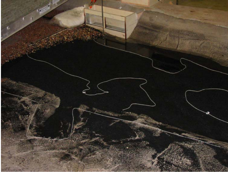
Photograph 11.—View of string contours of sediment deposited upstream of dam following steady-state flow of 4,000 ft 3 /s.
