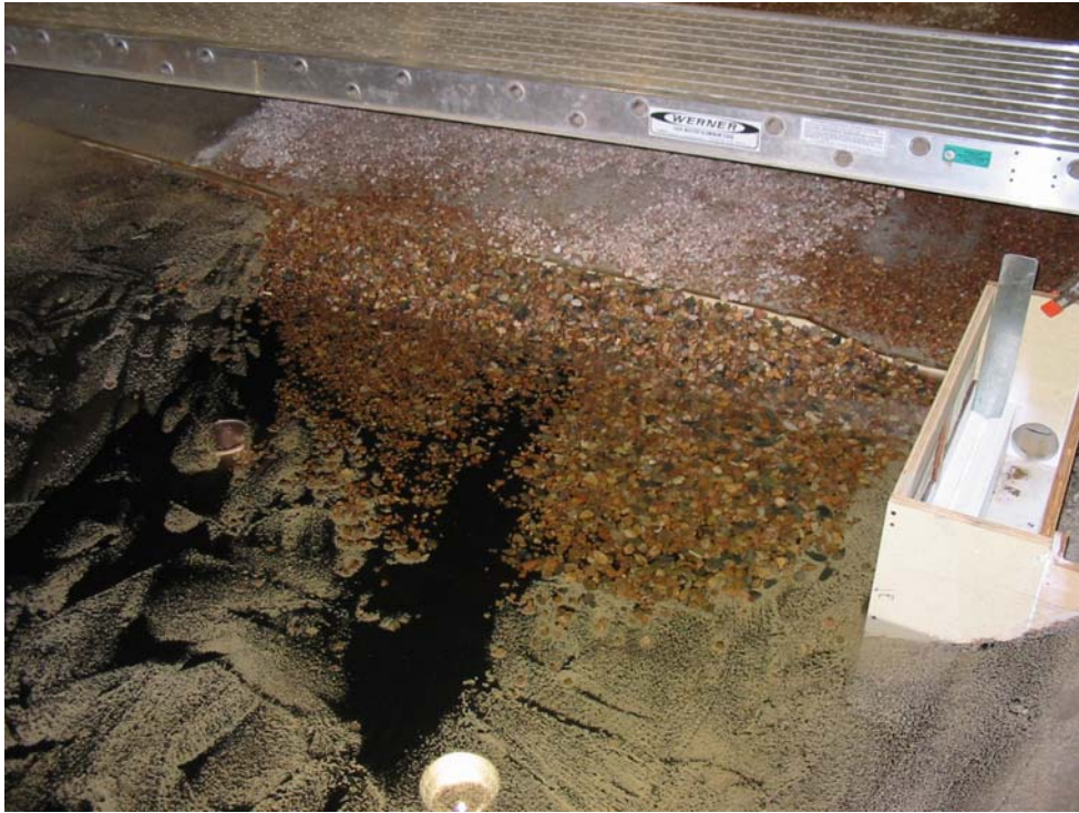
Photograph 7.—View of initial sediment deposit formation upstream of the dam during early stages of the alluvial bed building process.
