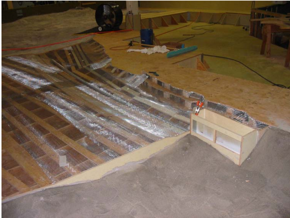
Photograph 3.—View of model construction showing intake structure and downstream rock-ramp.
