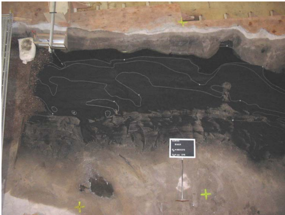
Photograph 15.—View of string contours of sediment deposited upstream of dam following 6,500 ft 3 /s peak flow hydrograph.
