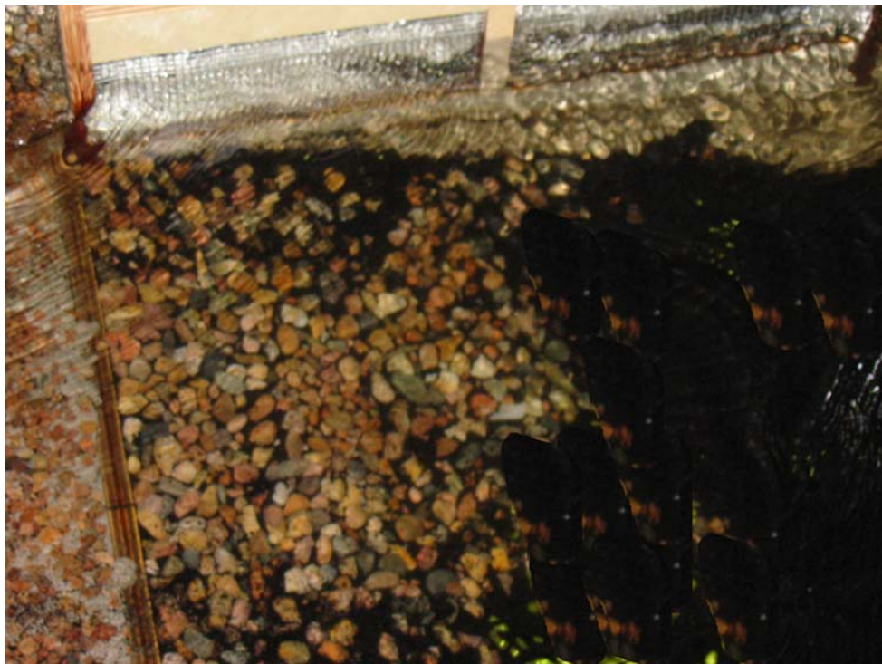
Photograph 8.—View of flow and bed sediment passing the front of the intake structure.
