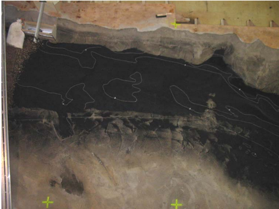
Photograph 12.—View of sediment deposited upstream of dam following steady-state flow of 4,000 ft 3 /s.
