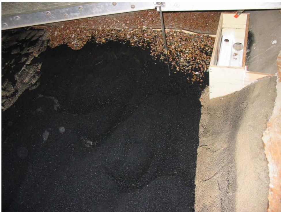
Photograph 10.—View of bed deposits upstream of dam crest following 4,000 ft 3 /s steady-state flow.
